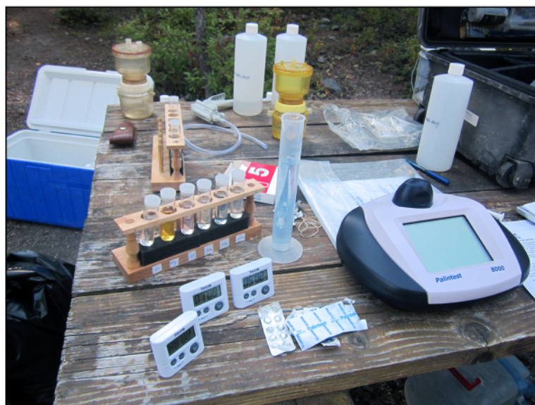
Figure 1. Photometer (lower right) and other instrumentation used in the proposed methodology. Photo by Ron Yehia.
