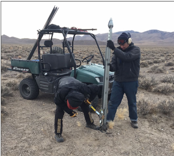
Figure 7. Shallow (2 m depth) temperature survey in southeastern Gabbs Valley.
