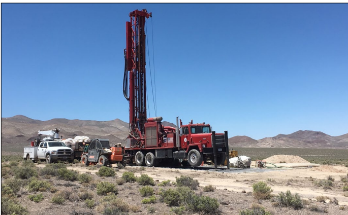
Figure 8. Temperature-gradient drilling in southeastern Gabbs Valley.
