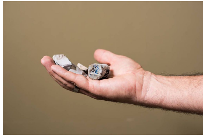
On the left, conventional cement shows the damage caused by harsh conditions found in power plants, geothermal wells, dams or in gas and oil applications. In contrast, PNNL's self-healing cement, on the right, could begin repairing itself within 24 hours of a crack appearing. Courtesy Andrea Starr, Pacific Northwest National Laboratory.
