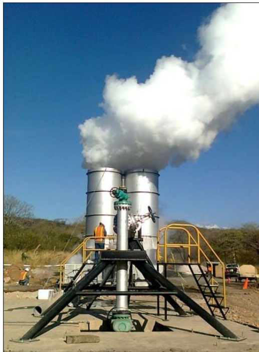
Flow testing of geothermal wells at the Mita Geothermal project. Courtesy Bluestone Resources.
