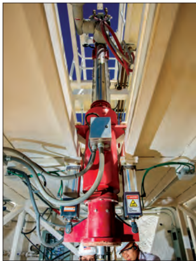
Technologist Elton Wright assists as mechanical engineer Jiann Su inspects a downhole hammer. PHOTO BY RANDY MONTOYA
