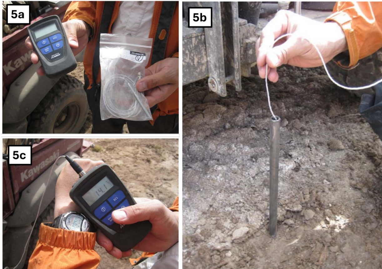
Figure 5. RTD and meter (a); Threading the RTD down the probe (b); and reading the temperature (c).
