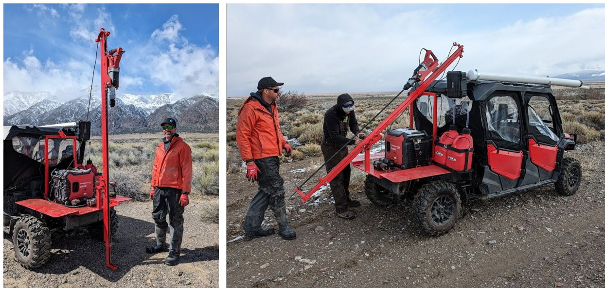
Figure 4. The 2 m probe rig designed and built for BPUS by Double R drilling.
