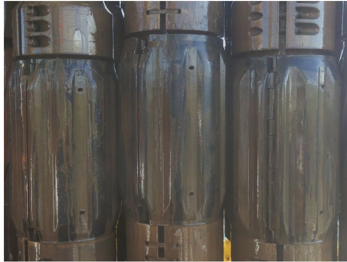
Figure 3: Improved high-temperature non-rotating protectors installed on drill pipe
