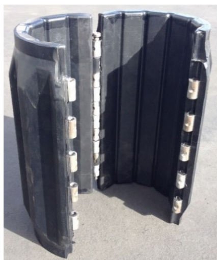
Figure 2: Improved high-temperature non-rotating protector sleeve with dual-hinge design
