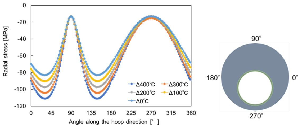
**Figure 10: Radial stress in the casing with 20% standoff for different temperature changes.**
