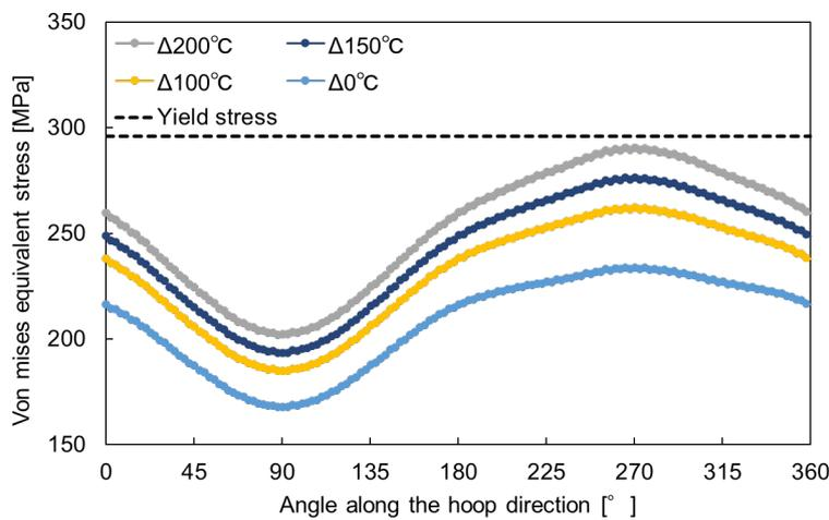
**Figure 12: The von Mises equivalent stress of casing with 20% standoff.**
