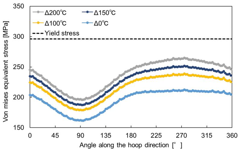
**Figure 13: The von Mises equivalent stress for a casing with 30% standoff.**
