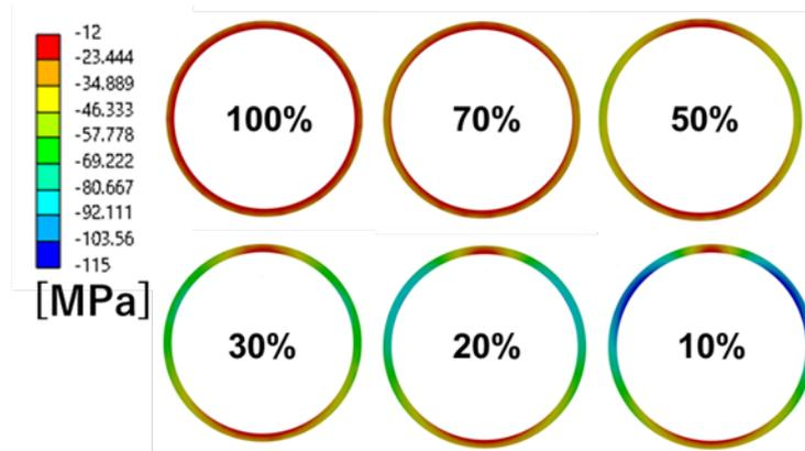
**Figure 7: Radial stress distribution in the casing for different standoff fractions.**
