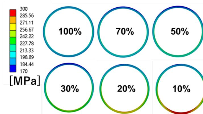
**Figure 8: The von Mises equivalent stress distribution in the casing for different standoff fractions.**
