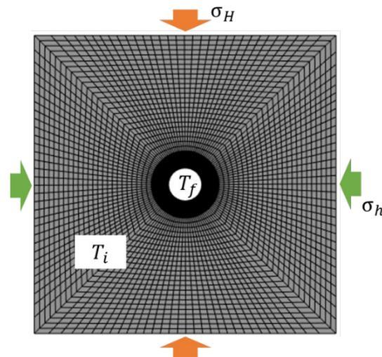
**Figure 5: Boundary conditions used for the finite element analysis. The maximum and minimum horizontal stresses  $\sigma_H = 83.8$  MPa and  $\sigma_h = 76.2$  MPa were applied at the model outer boundaries. The fluid temperature within the wellbore and the initial (formation) temperature are indicated by  $T_f$  and  $T_i$ , respectively.**
