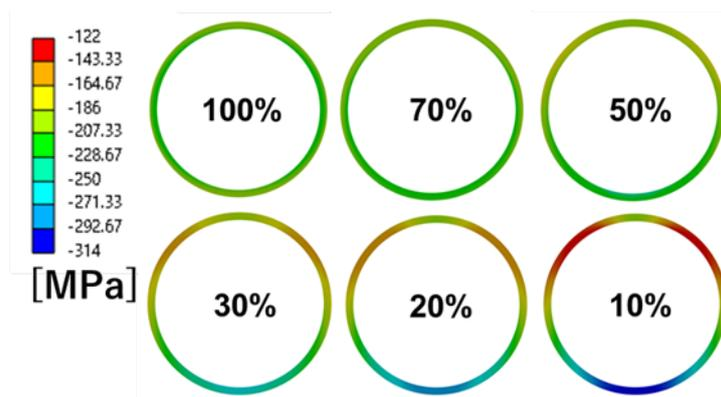
**Figure 6: Hoop stress distribution in the casing for different standoff fractions.**
