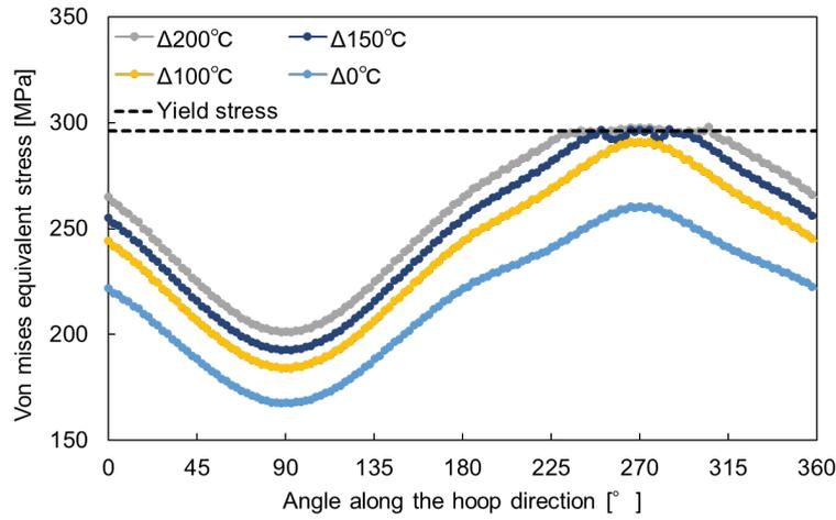
**Figure 11: The von Mises equivalent stress for a casing with 10% standoff.**
