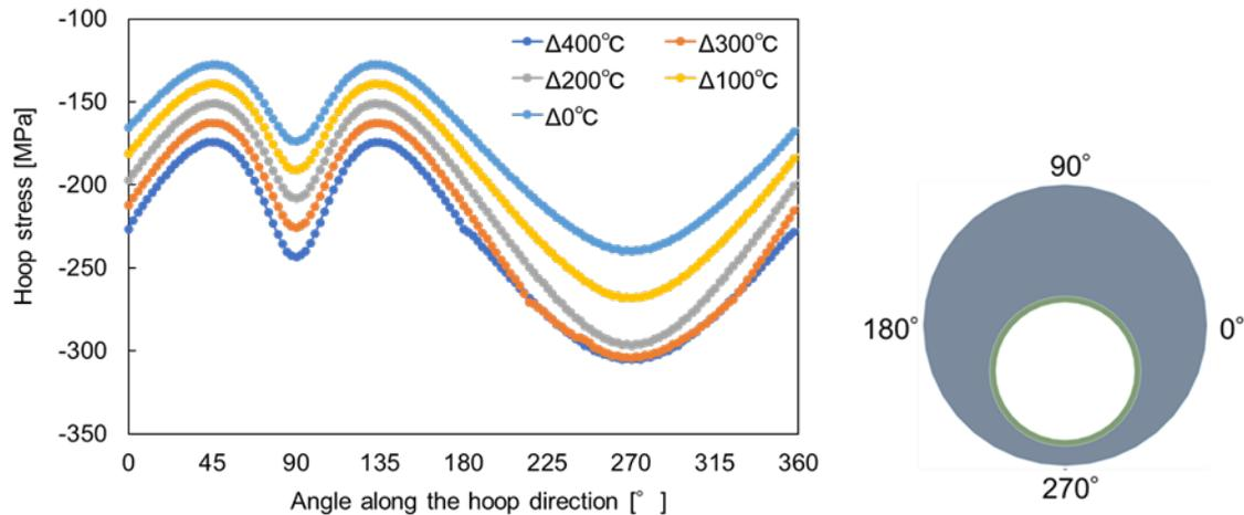
**Figure 9: Hoop stress in the casing with 20% standoff for different temperature changes.**
