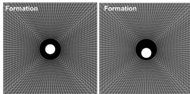
**Figure 3:** Mesh used in a 2D finite element model of a wellbore with (Left) a centered casing, and (Right) an eccentric casing.
