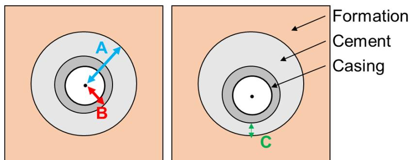
**Figure 2:** (Left) Centered well casing. (Right) Eccentric casing deviating from the center of the wellbore.
