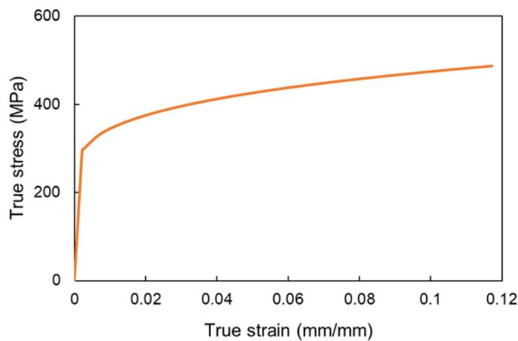
**Figure 4:** The stress-strain diagram of K55 grade casing at 500°C.
