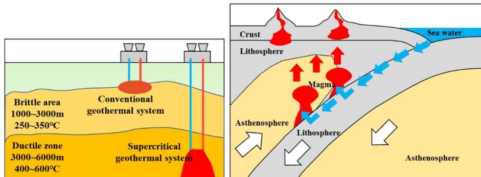
**Figure 1: (Left) Schematic diagram of a supercritical geothermal system. (Right) Example tectonic setting for a convergent plate boundary.**
