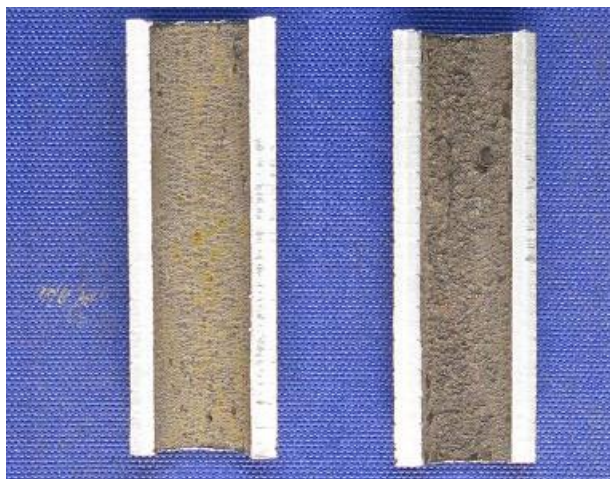
Figure 12. Internal condition of the inspection spool installed in the inlet stream.
