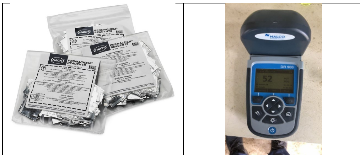
Figure 7. Hach® silica high range reagents and Hach® DR900 portable colorimeter were used to monitor the monomeric silica levels.
