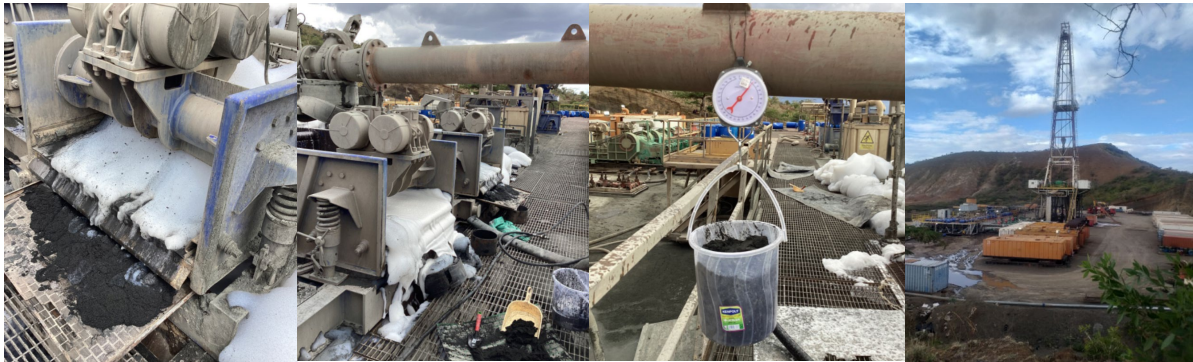
Figure 4: Data collection at well site during drilling at Paka geothermal field. The two images on the left show the shale shakers where the drill cuttings were collected. The third image shows the weighing of collected cuttings, and the rightmost image shows the drilling rig.
