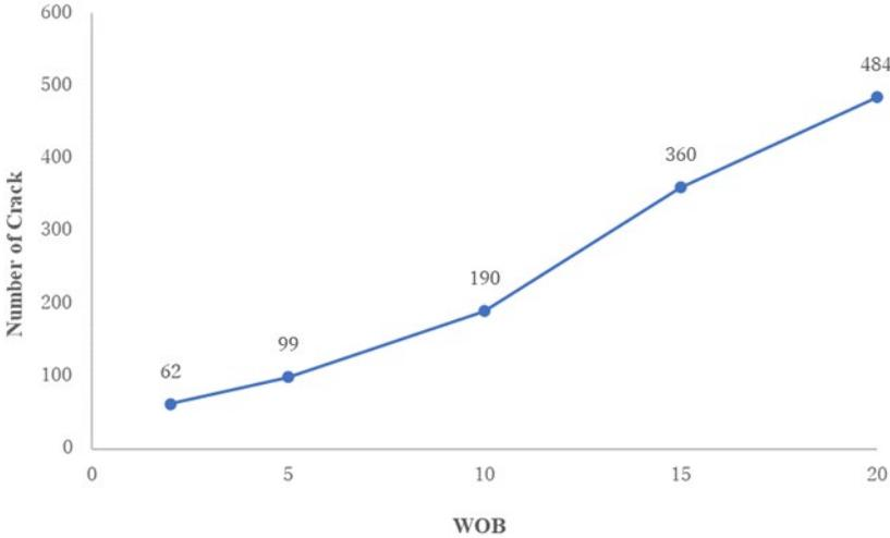
Figure 5: Number of cracks for each weight on bit (WOB).
