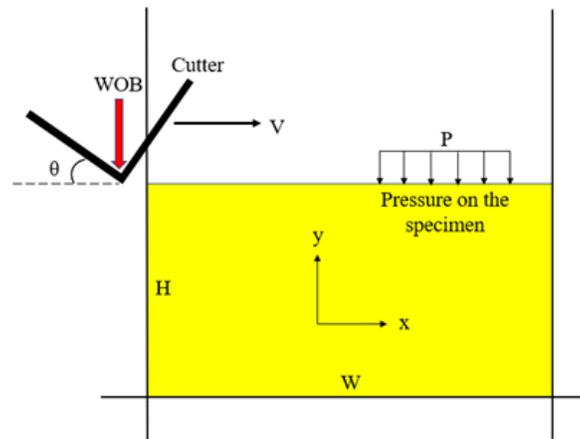
Figure 3: Schematic diagram of the rock cutting environment.
