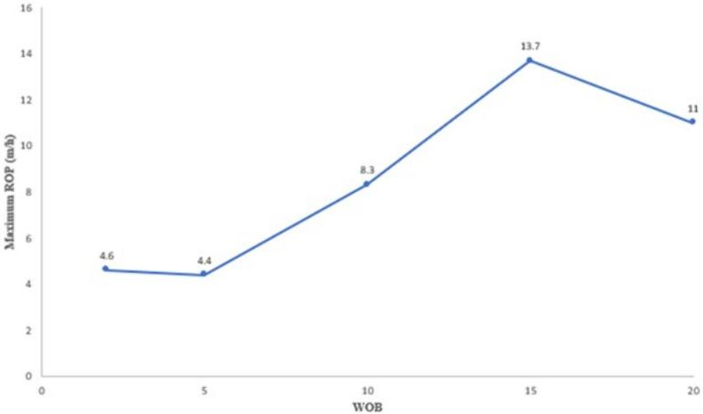
Figure 7: Maximum digging rate at each weight on bit (WOB).
