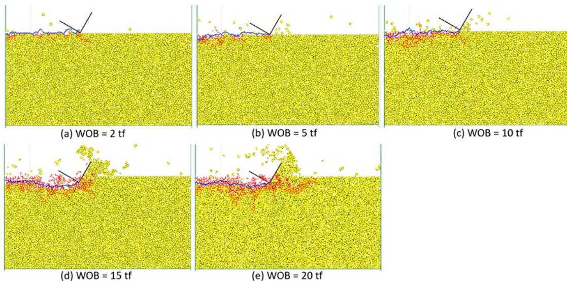
Figure 4: Cutting behavior and crack propagation.
