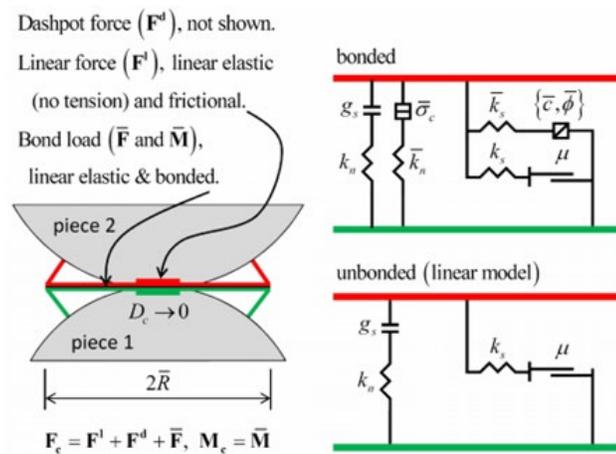
Figure 1: Schematic of the modified bonded particle model (Material-Modeling Support for PFC, 2021).
