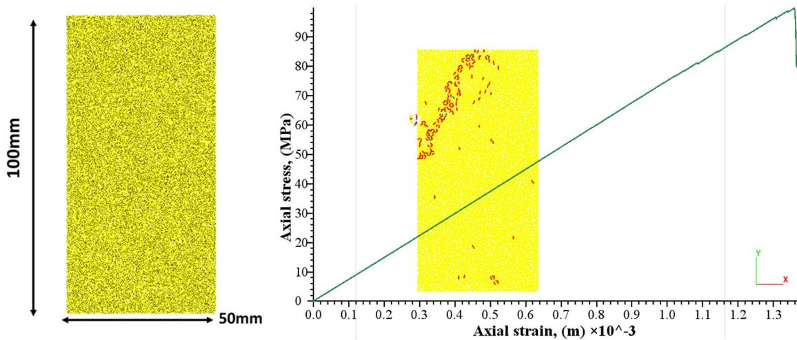
Figure 2: Rock grain model (left) and stress-strain diagram (right).
