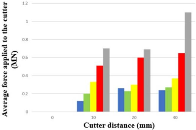
Figure 6: Average force to cutter vs. cutting distance.
