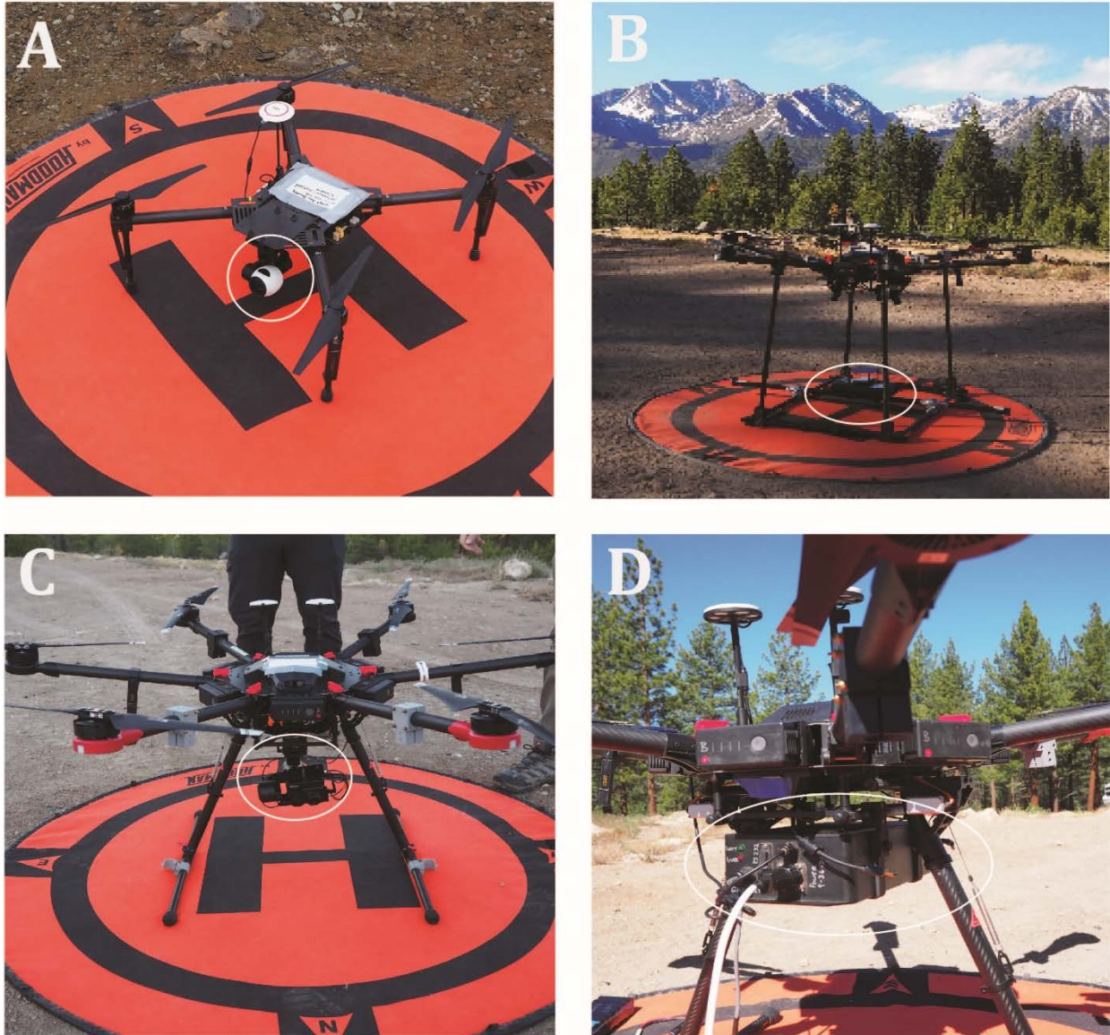
Figure 3: Photos of UAS platforms with payloads circled. (A) DJI Matrice 100 with Zenmuse X3 camera. Drone is 65-cm diameter. (B) DJI Matrice 600 Pro with Sensys MagDrone R3 magnetometer on carbon fiber frame. Drone is ~1.6-m diameter. (C) DJI Matrice 600 Pro with FLIR Duo Pro R thermal camera, mounted on a Gremsy S1 V3 gimbal. (D) DJI Matrice 600 Pro with U.S. Geological Survey UAS Multi-GAS instrument. Photographs by Jonathan Glen, U.S. Geological Survey.
