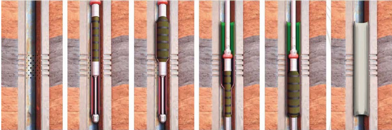
Figure 2: Patch setting sequence
