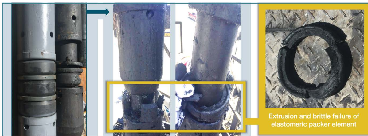
Figure 8: A packer for use in zonal isolation is a clear case study of elastomeric failure, seen here before and after downhole deployment. The “shoulder” produced by seal extrusion is a clearly visible pain-point for EGS well operation. Images courtesy of Prof. John McLennan.
