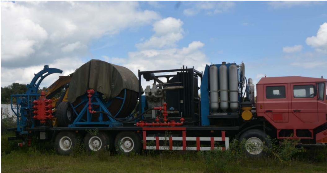
Figure 3: Coiled tubing truck with all equipment
