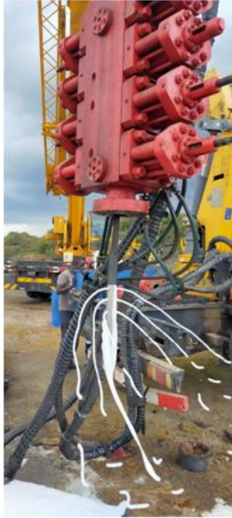
Figure 8: Testing the lead tool before running coiled tubing in hole
