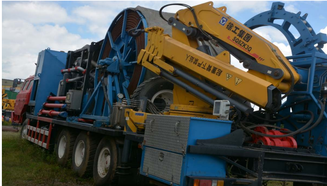
Figure 4: Coiled tubing truck showing position of crane and control console
