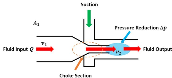
**Figure 1: Principle of the Venturi effect.**
