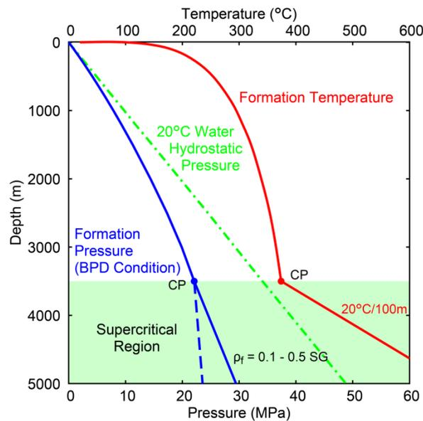
Figure 3: Assumed pressure and temperature profiles of supercritical geothermal drilling (Naganawa, 2017).
