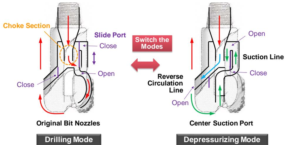
Figure 2: Concept of the Thermal-Shock Enhanced (TSE) Drill Bit (Naganawa, 2018).
