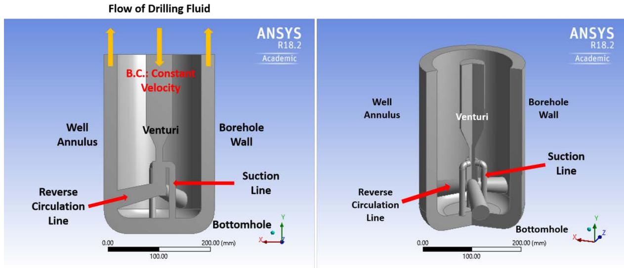
Figure 5: Simplified model setting of the flow areas inside and around the thermal-shock enhanced drill bit.
