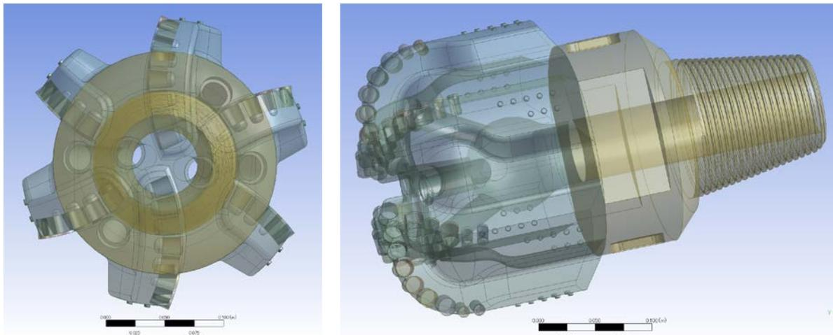
Figure 4: Original 3D model of 8 1/2-in. PDC bit used in this study.
