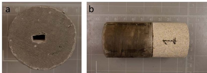
Figure 2. a) Slit made in cement plug, by positioning a silicon mold and pouring the cement slurry around it. b) Cement plug glued to Castlegate outcrop sandstone, serving as filter for hydraulic integrity testing.
