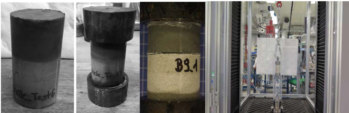
Figure 1. From left to right: composite shale-cement plug, the same plug glued to the load-frame metal cups, fracture between sandstone and cement after testing, and chain rig for tensile testing in load frame.
