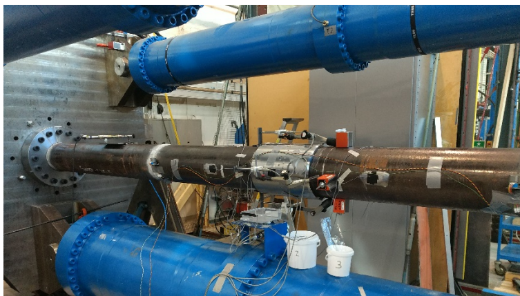
Figure 2: Test setup for testing 9 5 / 8 " Flexible Coupling in SINTEF laboratories in Norway.
