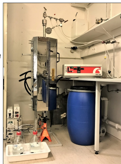
Figure 2: The laboratory setup of the flow-through reactor.
