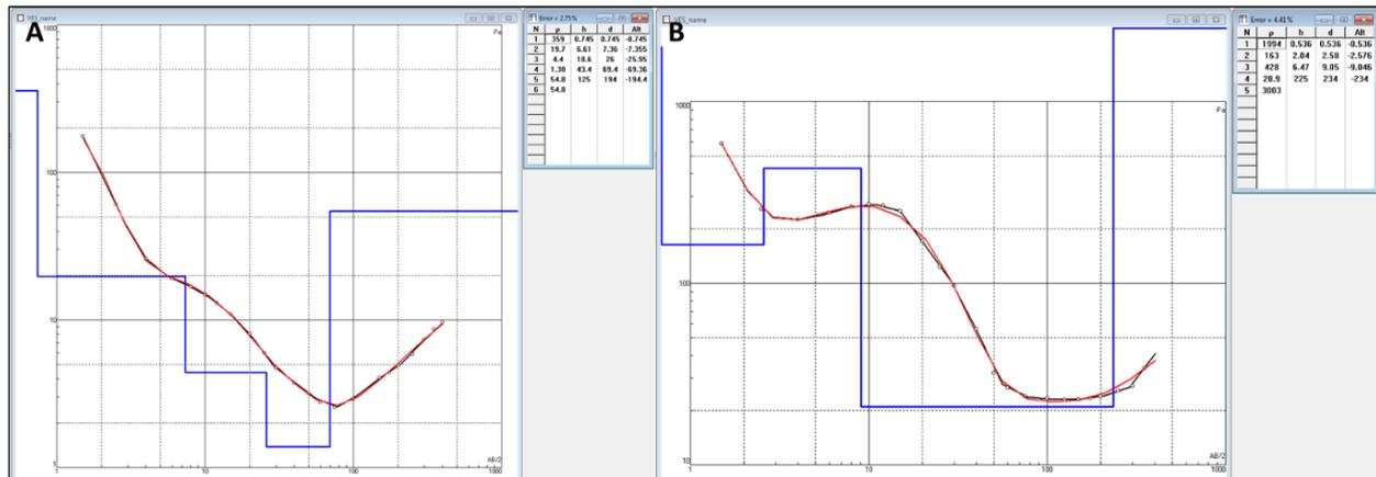
Figure 2. The A and B image represent 1D models of layers from the interpretation of the VES.
