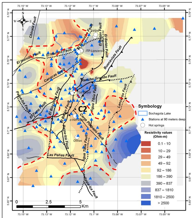
Figure 4. Demarcated area at 90 meter deep where the conductive responses with lateral continuity are concentrated.
