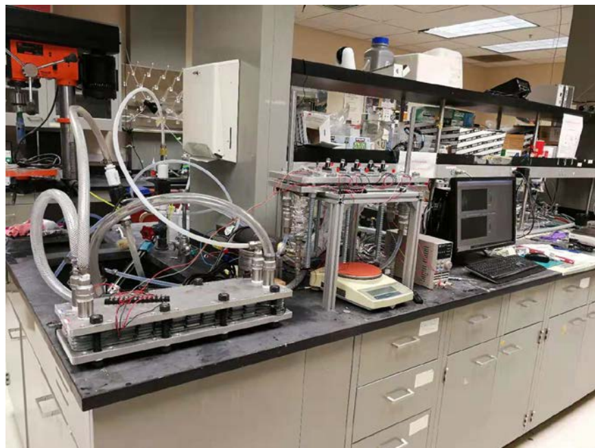
Figure 4: Photo of the lab-scale thermoelectric power generation system.
