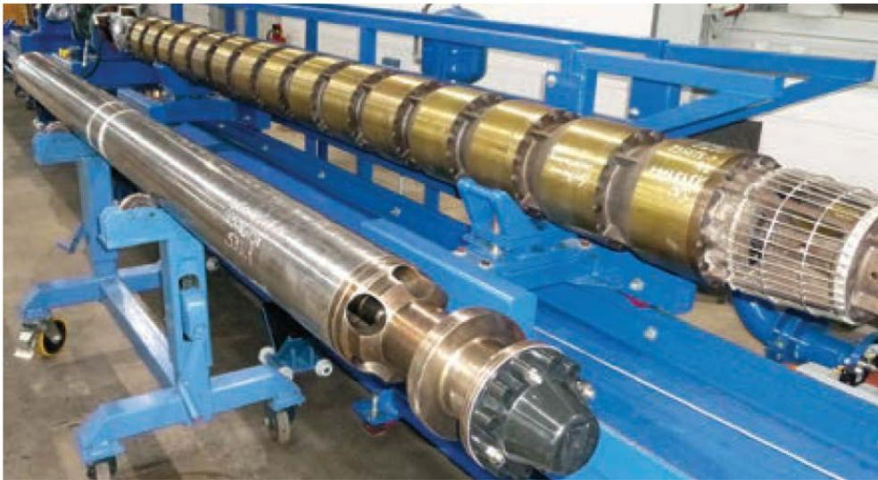
**Figure 2: A bolted bowl pump, top/right (~3200GPM, 200 l/s) compared to a smaller housed pump, bottom/left (~1600GPM, 100 l/s)**
