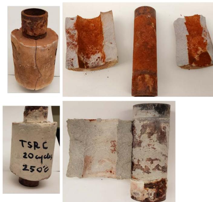
Figure 4. Appearance of OPC/SiO<sub>2</sub> sheath samples (top) and TSRC sheath samples (bottom) after 20 severe TS cycles
