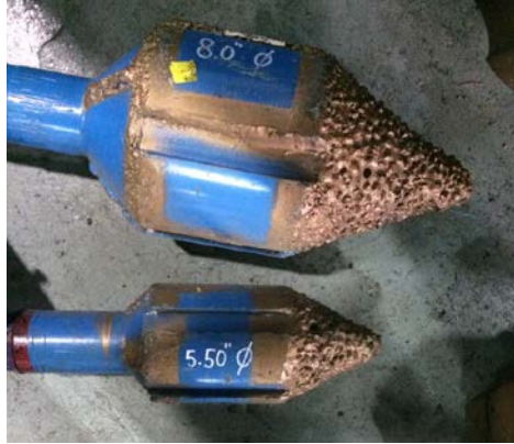
Figure 6: Photos of the tapered mill used at AWI A-4
