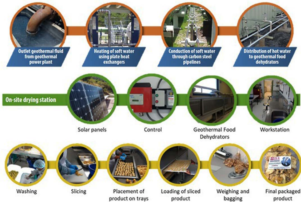
Figure 6 Process Description of Geothermal Food Dehydrator
