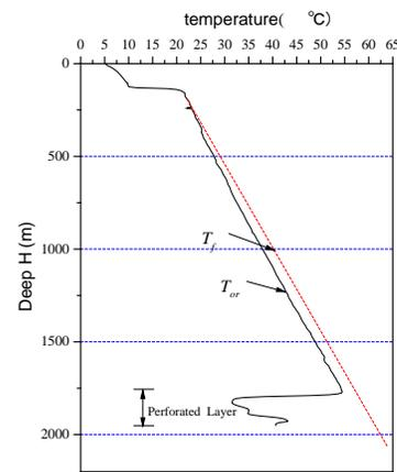
Figure 2: Temperature-depth profile of water in the test well
