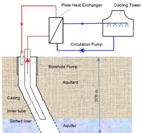
Figure 1: Schematic test system of DDHE
