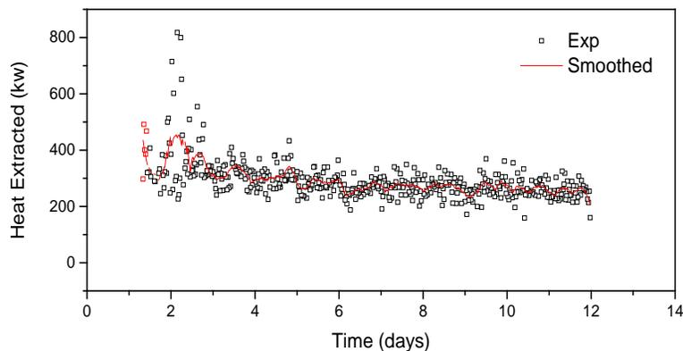
Figure 4: The heat extraction of the DDHE with time
