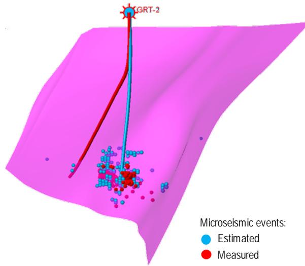
**Figure 3: Geomechanical simulation results: simulated and measured microseismic events during the injector well stimulation. The main fault crossing the site is shown in the background (From Sosio et al., 2018).**
