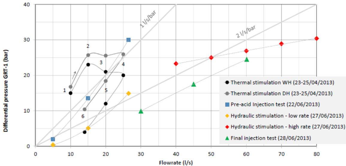
Figure 2: Injectivity evolution of GRT-1 during the different injections (from Baujard et al., 2016).
