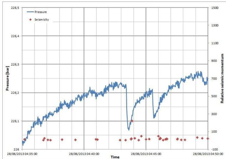
Figure 5: Two examples of pressure drops and their associated burst of seismicity at Rittershoffen (Meyer et al. 2017).
