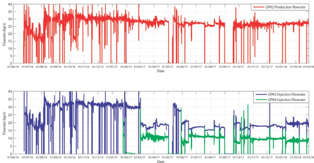
**Figure 6: Production flowrate from GPK2 (red curve), injection flowrate in GPK3 (blue curve) and GPK4 (green curve) between June 2016 and September 2017.**
