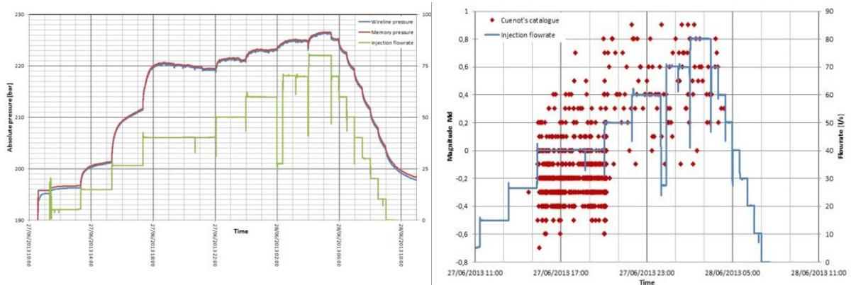
**Figure 4: Left: Pressure data recorded by the wireline sensor (blue) and memory (red). As they are very similar, the catalogue with the smallest time step has been chosen (Baujard et al., 2017). Right: MP catalogue of induced seismicity during the hydraulic stimulation (Meyer et al., 2017).**
