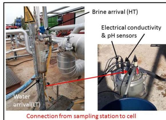
**Figure 8: Sampling cell and sensors**
