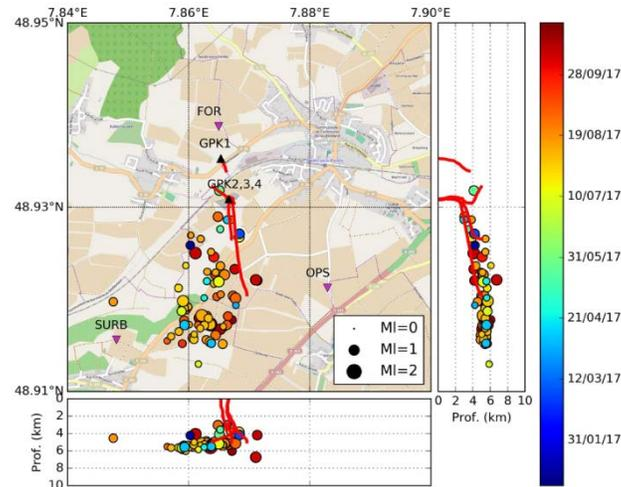
**Figure 7: Induced seismicity located around GPK-4 in 2017.**
