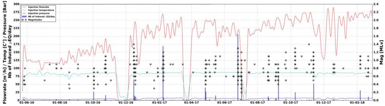
Figure 10: Moving average of injection flowrate values (red curve), injection temperature (light blue curve), injection pressure (dark blue curve) and associated microseismic events local magnitudes (points, right scale) in Rittershoffen heat plant between June 2016 and March 2018.
