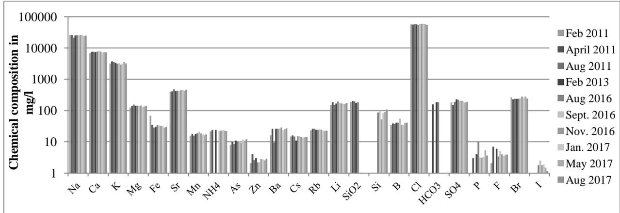
Figure 9: Elementary chemistry from geothermal brine - GPK2 (Mouchot et al., 2018)
