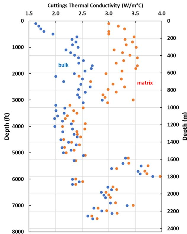
**Figure 7. Thermal conductivity data for well 58-32 based on cuttings measurements using a divided bar. Matrix thermal conductivity values are corrected for the effects of rock porosity using the wireline geophysical logs (formation density log; Gwynn, 2018). The variation in thermal conductivity is largely due to the quartz content of the rock. The transition from granitic basin fill to granitic bedrock occurs at 1000 m.**
