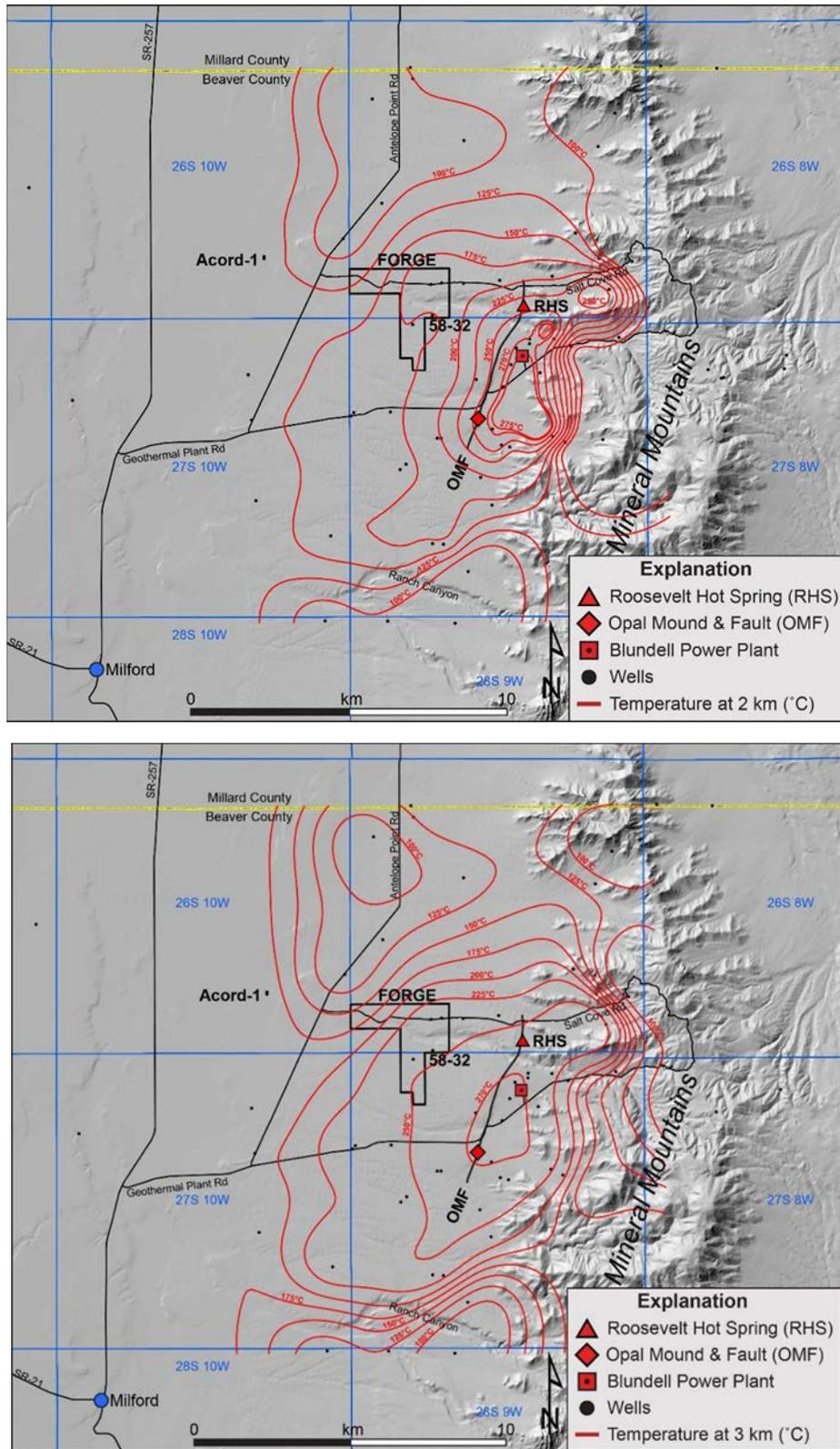
Figure 9. Isotherm maps at 2 and 3 km depth based on analysis of the temperatures in thermal gradient wells and deeper exploration wells.
