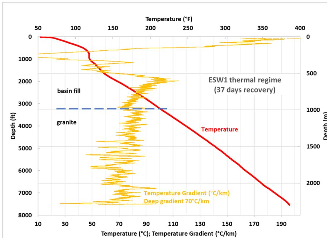
**Figure 6. Thermal profile in 58-32 37 days after drilling and testing stopped. The temperature gradient near the bottom of the well of  $70^{\circ}\text{C}/\text{km}$  is probably close to the deep, equilibrium conductive gradient at this site. The increased gradient between 1500 and 500 m depth is suspected to be an artifact of non-thermal equilibrium. The near isothermal section between 200–300 m depth indicates a groundwater aquifer.**
