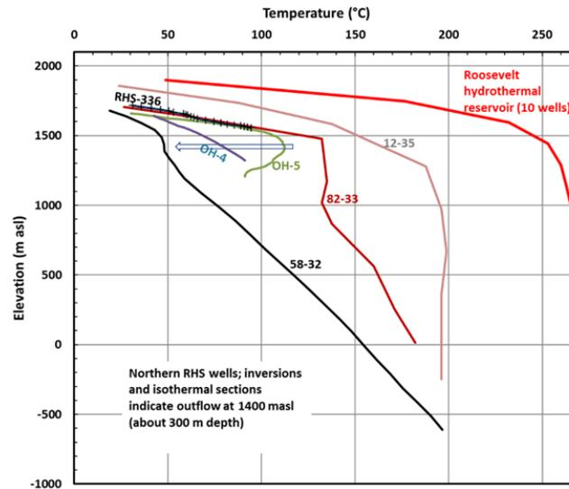
Figure 3. Temperature profiles in wells around the northwest of RHS system where the main outflow zone of hot water occurs. The outflow is characterized by temperature inversions (OH-5) and isothermal zones between 1500 and 1700 m asl (typically 200–400 m depth; blue arrow). 58-32 was drilled during Phase 2B of the FORGE project.
