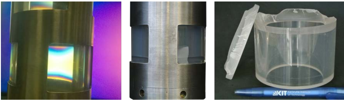
Figure 4: Result of a gluing joint between the cylindrical side window and Inconel ® 718 housing; left: stresses visualized by polarized light; center: fracture of the side window after an autoclave test; right: removed ceramic side window with fracture after stress test
