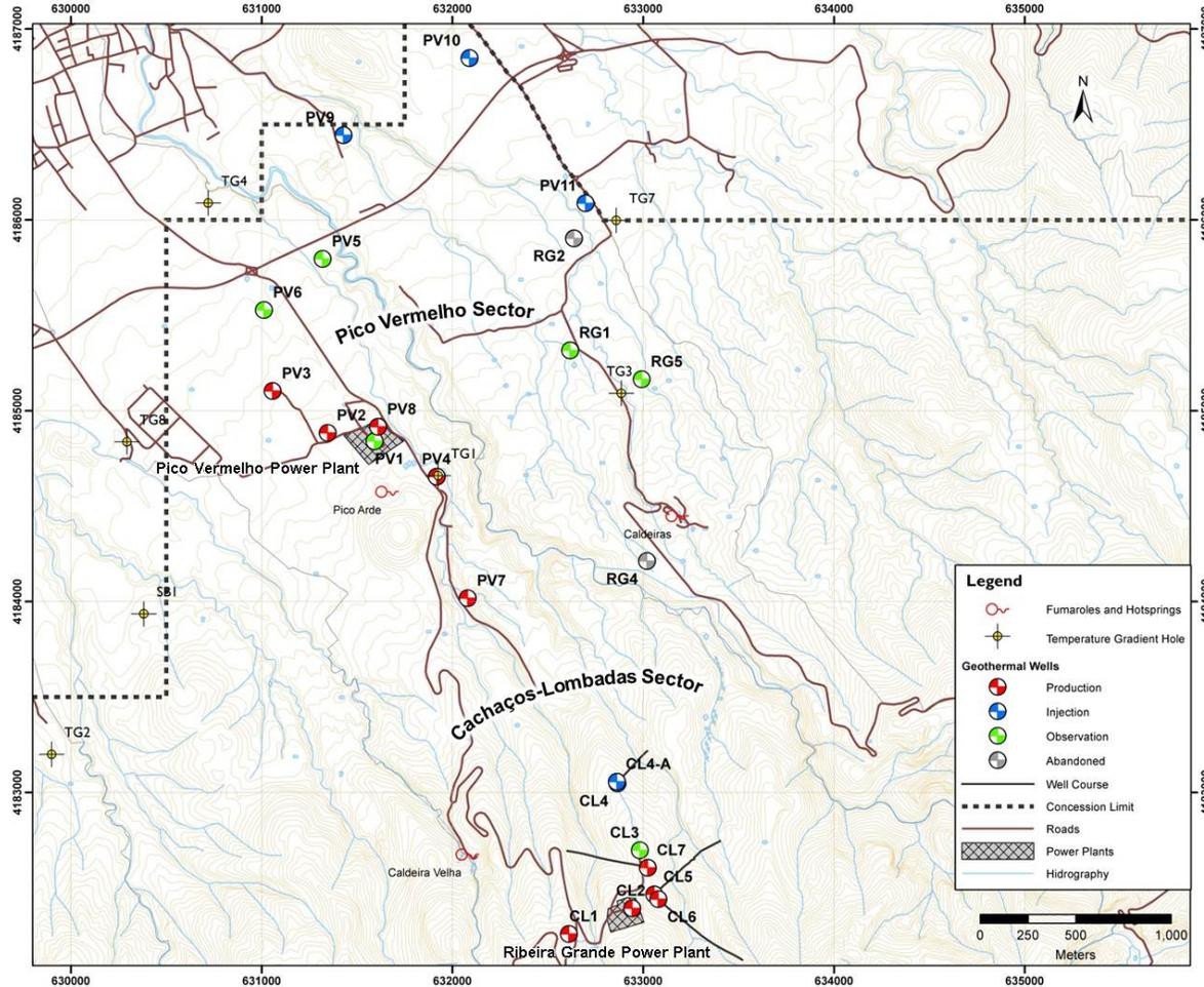
**Figure 3: Ribeira Grande geothermal field. Datum WGS 84, Zone 26S (EDA Renováveis, S.A.).**
