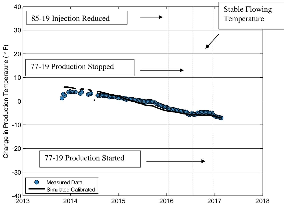
**Figure 8: 88-19 Measured and Simulated Change in Production Temperature**
