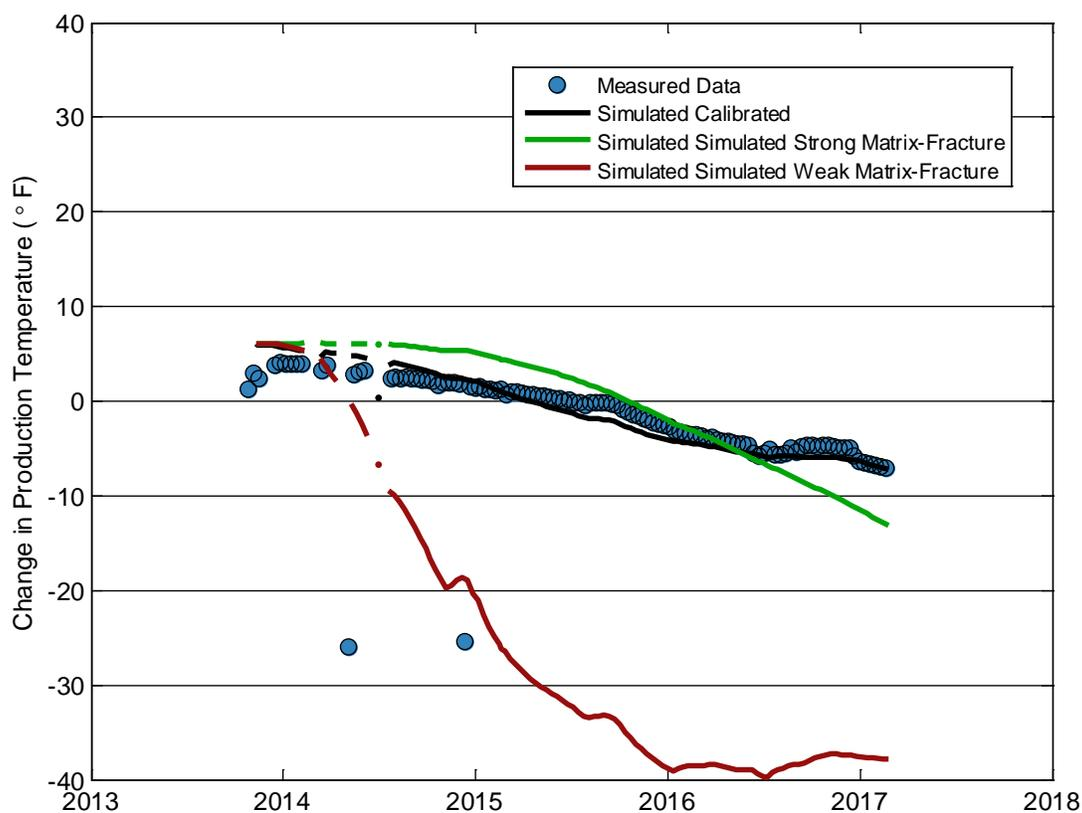
**Figure 9: 88-19 Measured and Simulated Change in Production Temperature**
