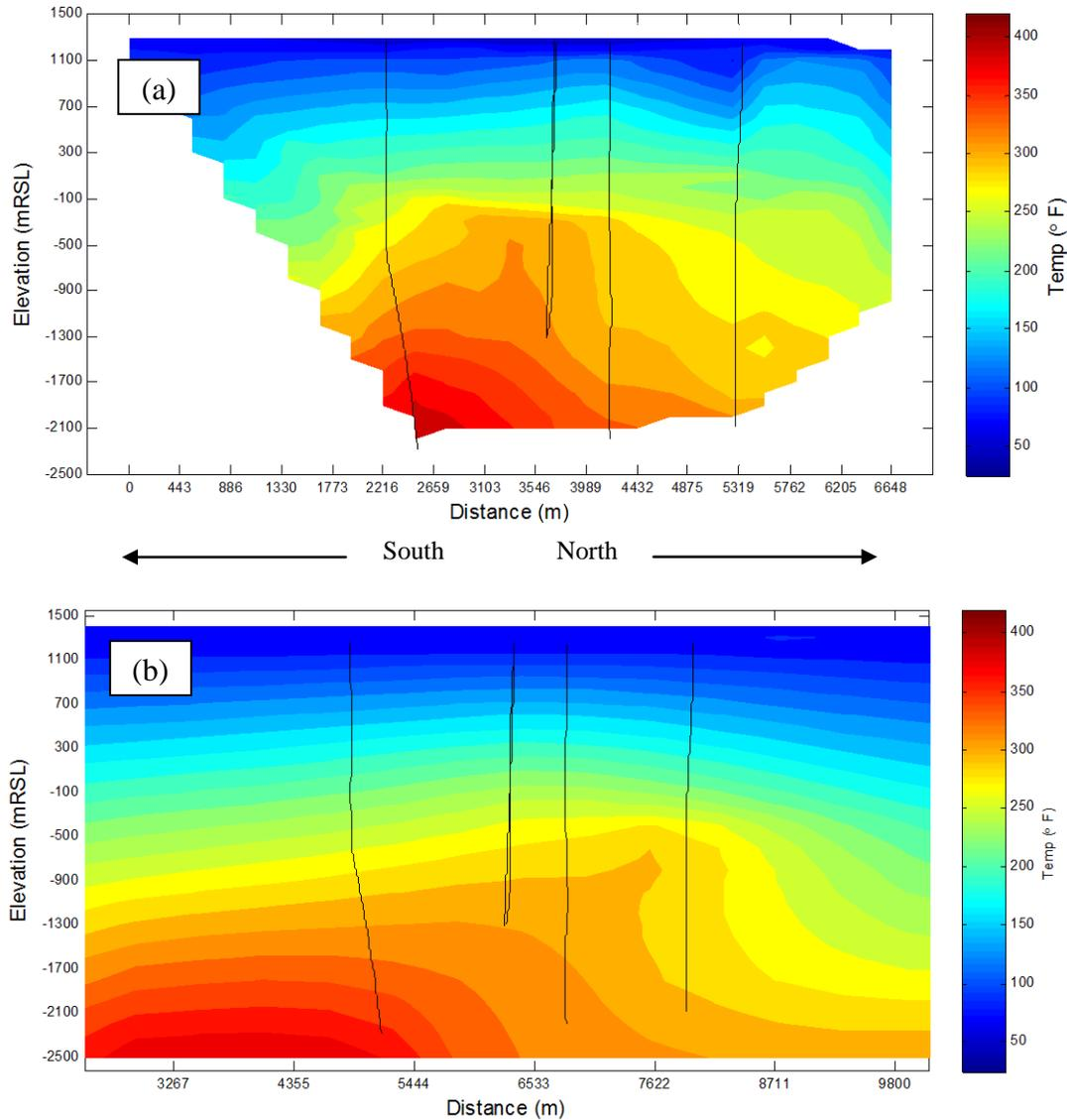
**Figure 5: Measured (a) and Simulated (b) Natural State Temperature Contours on Faults Zone 2**
