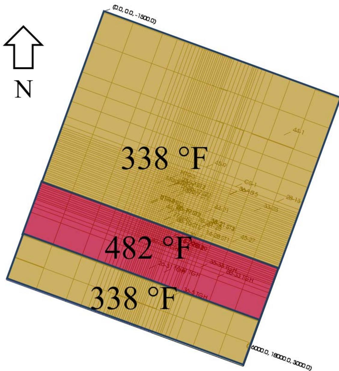
Figure 4: Constant Temperature Boundary Conditions on Model Bottom
