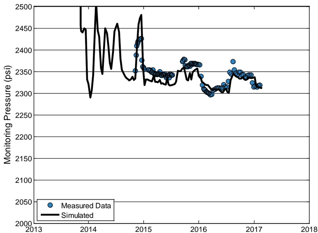
**Figure 7: Fault Zone 2 Measured and Simulated Monitoring Pressure**
