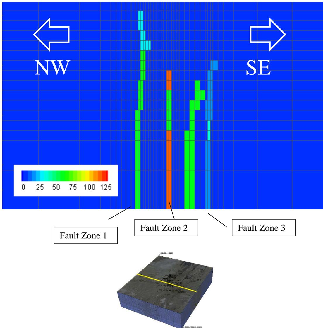
**Figure 2: Vertical Slice of Numerical Model Total Permeability. View from Southwest (Slice Location Shown)**
