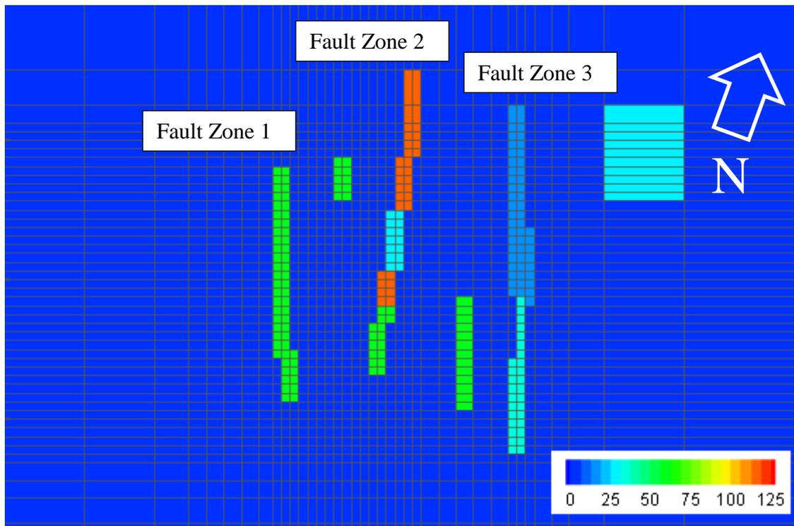
**Figure 1: Horizontal Slice of Numerical Model Total Permeability in millidarcies at -1200 mRSL
