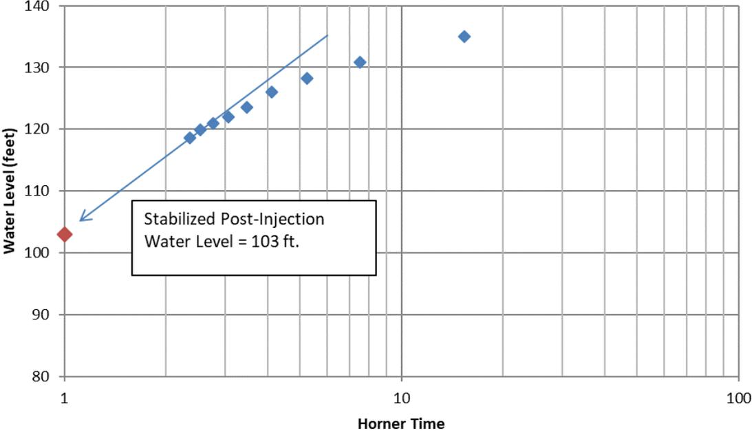
Figure 7: Horner plot approximation for stabilized post-injection water level
