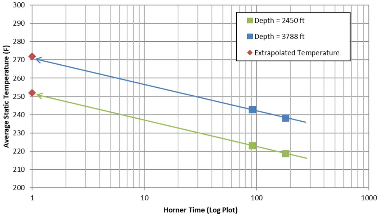
Figure 9: Horner analysis on temperature buildup
