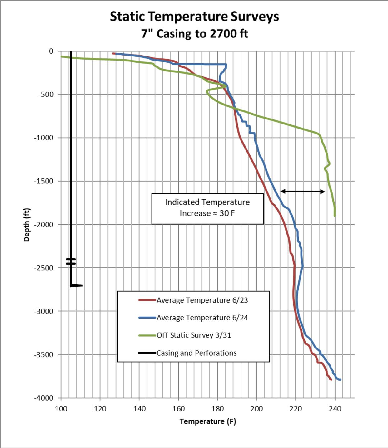
Figure 8: Static temperature surveys showing heat up
