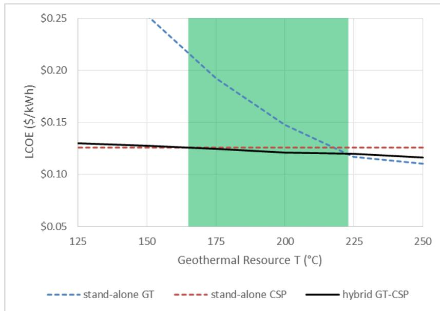
**Figure 2. Undiscovered Hydrothermal LCOE for stand-alone binary GT, stand-alone CSP, and hybrid CSP-GT power plants in Business-As-Usual Scenario. The LCOE for the hybrid plant is lower than the LCOE for both stand-alone GT and CSP plants in the range of geothermal resource temperatures designated by the shaded plot area.**
