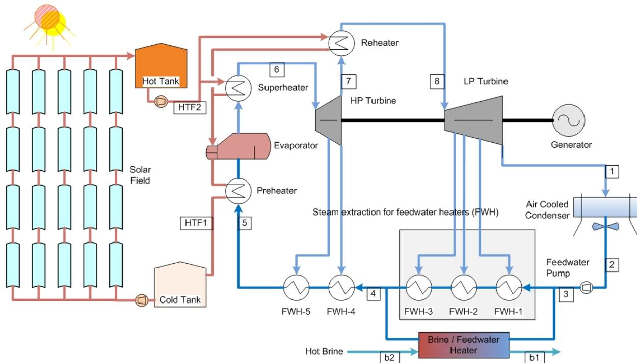
**Figure 1. Schematic of a representative CSP plant showing energy from geothermal brine replacing the three low-temperature feedwater heaters (FWH-1, FWH-2, and FWH-3), thereby eliminating steam extractions from the low-pressure turbine. Open, hot (direct contact) FWHs are shown for simplicity, although the model uses closed FWHs (Turchi et al., 2014).**
