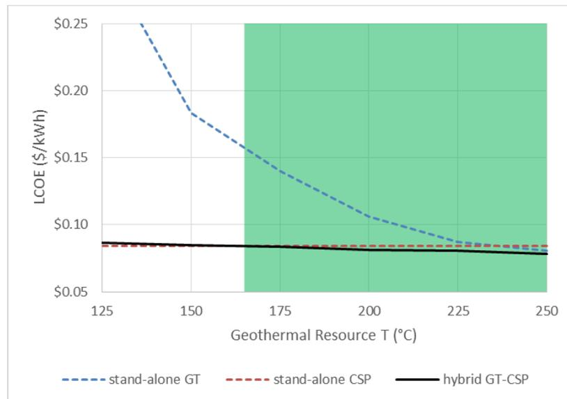
**Figure 3. Deep EGS LCOE for stand-alone GT, stand-alone CSP, and hybrid CSP-GT power plants in Exploration De-Risk Scenario. The LCOE for the hybrid plant is lower than the LCOE for both stand-alone GT and CSP plants in the range of geothermal resource temperatures designated by the shaded plot area.**
