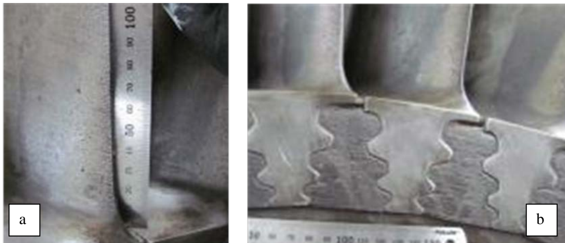
Figure 4: a) Trailing edge erosion and b) water wash erosion on rotor blade root fixing.
