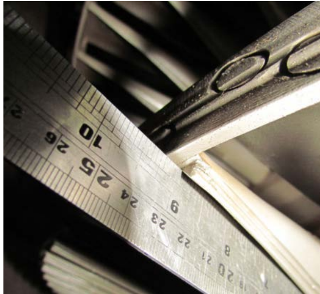
Figure 7: Groove cut into coverband by diaphragm seal
