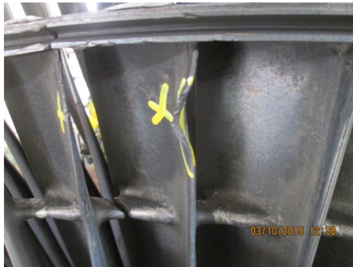
Figure 5: Damage from “domestic” object seen on leading edge of rotating blade.
