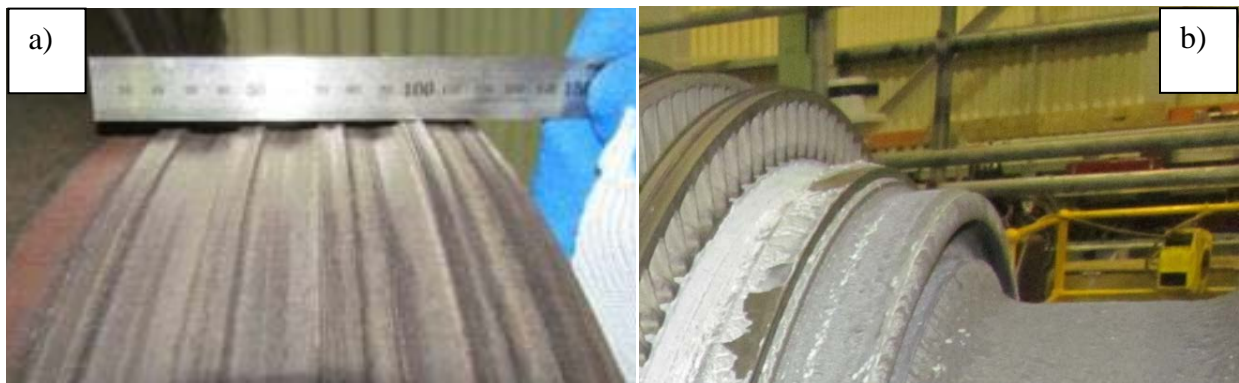
Figure 6: a) Solid particle erosion found on gland seals. b) Scale (silica) formation
