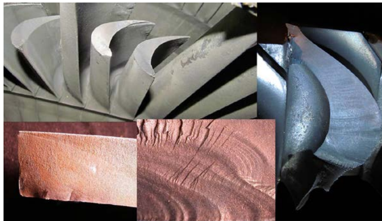
Figure 8: Typical locations and appearance of fatigue fractures.
