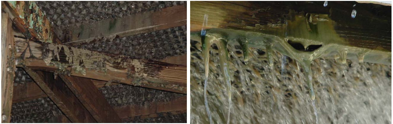
Figure 8. Detachment of biofouling deposits during 28-day evaluation program in CP IV Unit #12.
