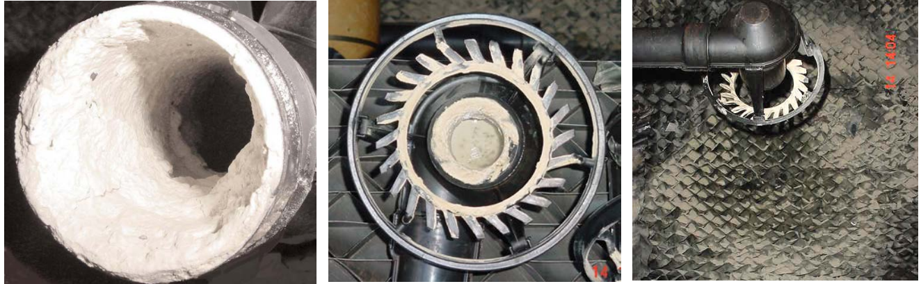
Figure 4. Sulfur fouling of distribution lines (left), spray nozzles (center) and tower fill (right).
