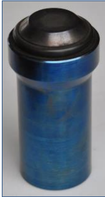
Figure 32. Check valve tempering temperature color change
