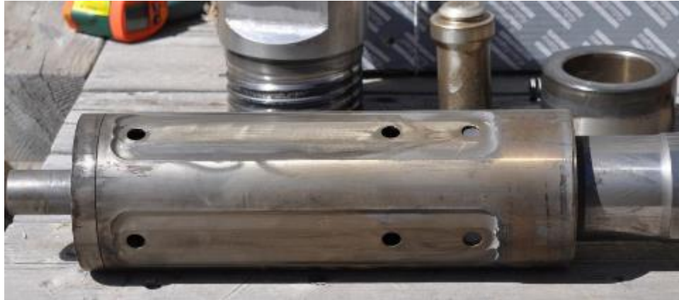
Figure 22. Piston sleeve assembly after operating at 400°F
