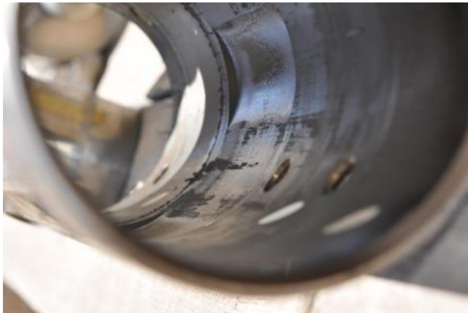
Figure 23. Piston sleeve inner diameter after operating at 400°F
