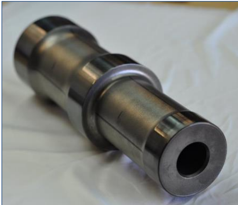
Figure 26. LT piston with DLC coating applied
