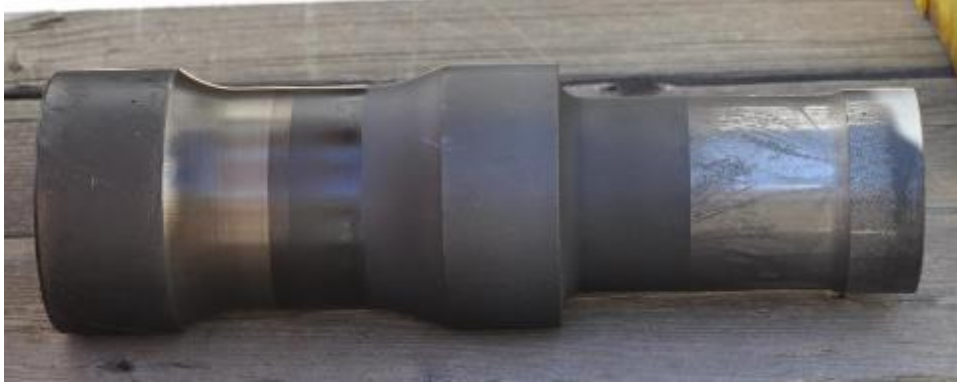
Figure 24. Piston with no lubrication at 400°F
