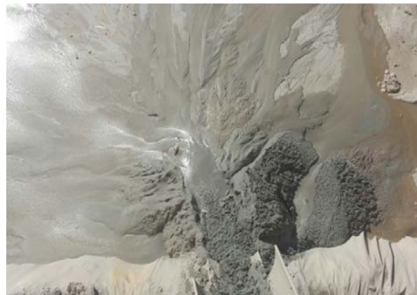
Figure 11: The figure above is the cavings and cutting samples while reaming in mud pit
