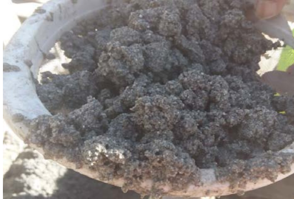
Figure 10: The figure above is the cavings and cutting samples while reaming
