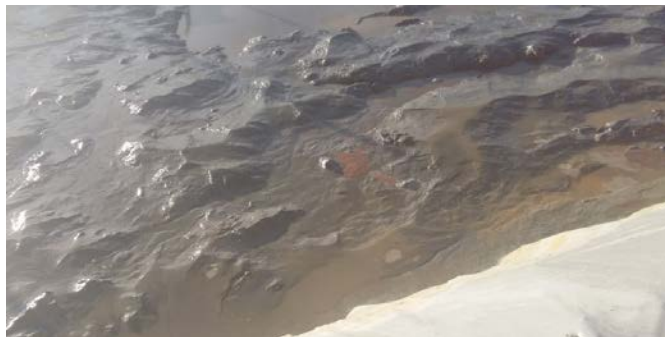
Figure 8: The figure above is the clay sized cuttings in mud pit cuttings during the cleaning flow
