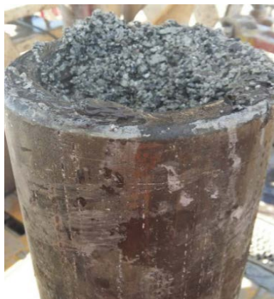
Figure 7: The figure above is the formation cuttings inside the drill collars
