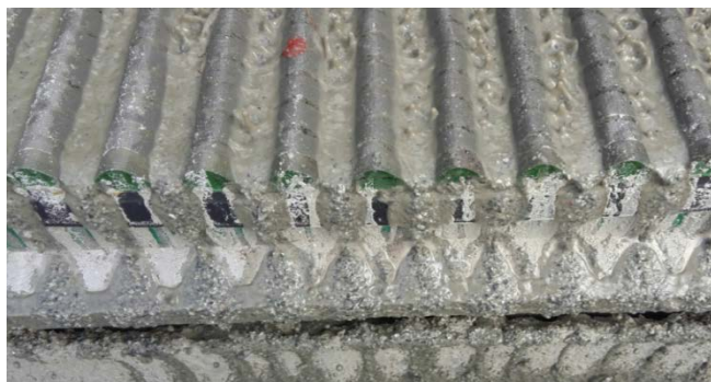
Figure 9: The figure above is the formation cuttings on shale shakers while circulating at 9 5/8" casing shoe
