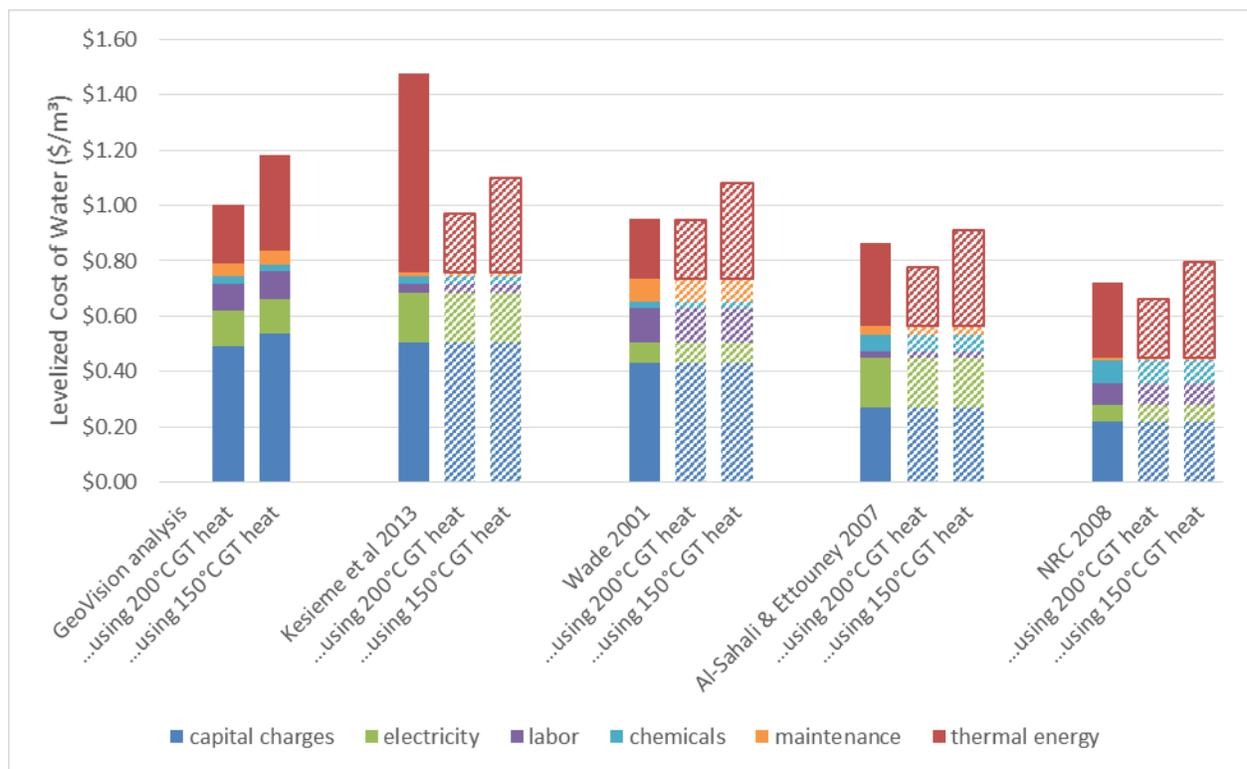
**Figure 6. Cost breakdown for several MED thermal desalination cost analyses (Kesime et al 2013 costs based on 20,000 m<sup>3</sup>/day capacity without use of waste heat). The second and third columns in each set substitute thermal energy costs corresponding to use of 200°C and 150°C hydrothermal resources in the Exploration De-Risk Scenario.**
