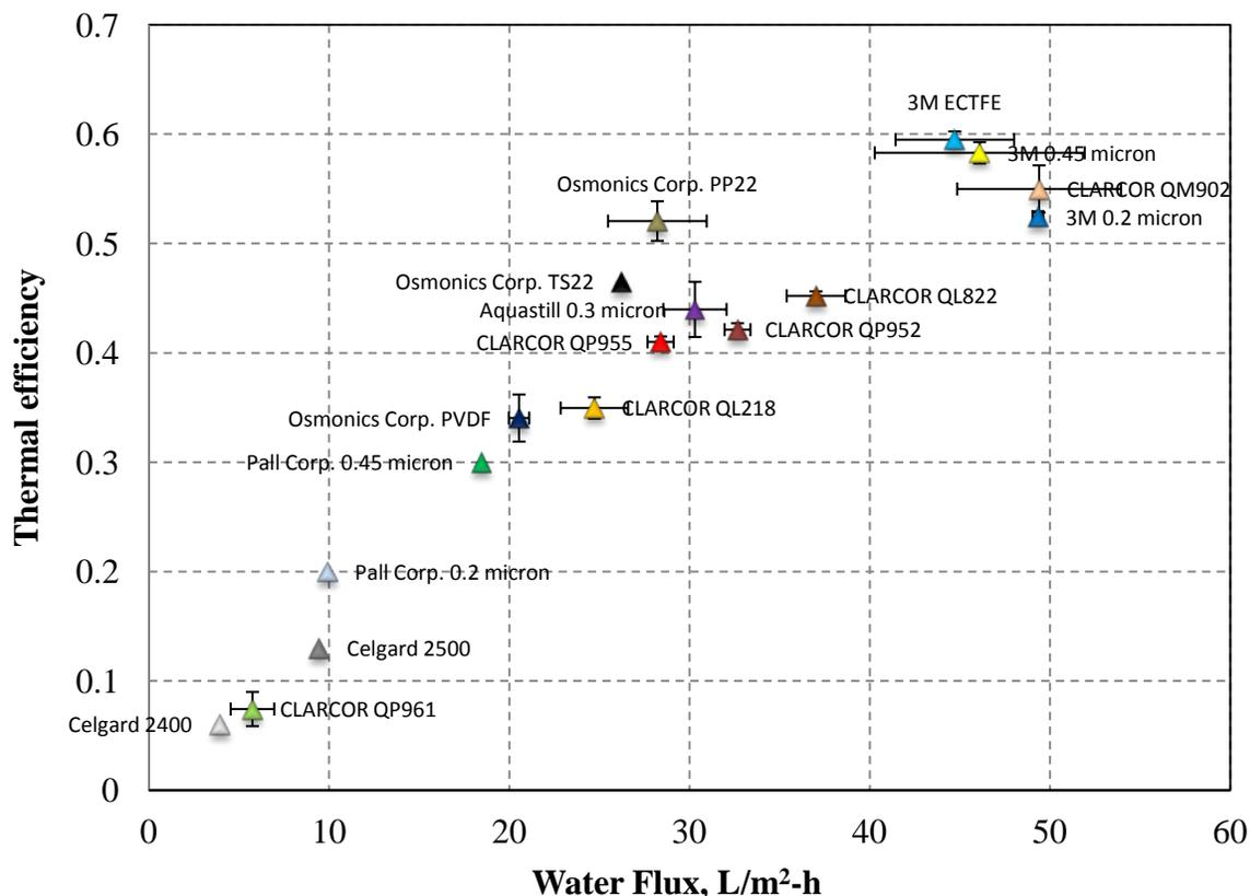
Figure 2. Thermal efficiency versus water flux for the different membranes. Feed and distillate temperature of 60 and 20 °C respectively. Feed and distillate flow rate of 1.6 LPM. Feed concentration of 1 g/L NaCl. Standard deviation is based on three different samples.
