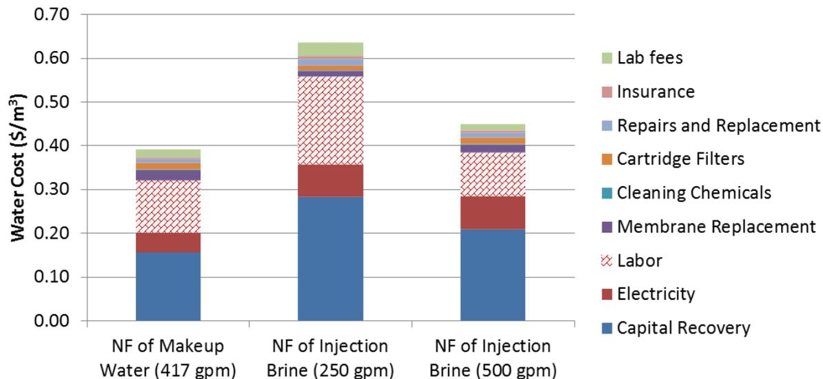
**Figure 5. Overall estimated cost of water for NF treatment of the makeup or injection brine flows. MD costs for a comparable flow rate of distillate (250 gpm) was estimated at  $\$1.60/\text{m}^3$  and was considered noncompetitive.**
