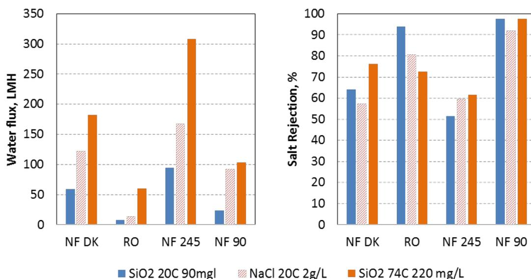
**Figure 3.** Water flux (left) and NaCl rejection (right) for NaCl solution and two silica/NaCl solutions at two different temperatures. Tests run at 150 psi to match the injection brine pressure. The NaCl pre-compaction test was operated at 300 psi. Cross flow was 1 LPM and membrane area 139 cm<sup>2</sup>.
