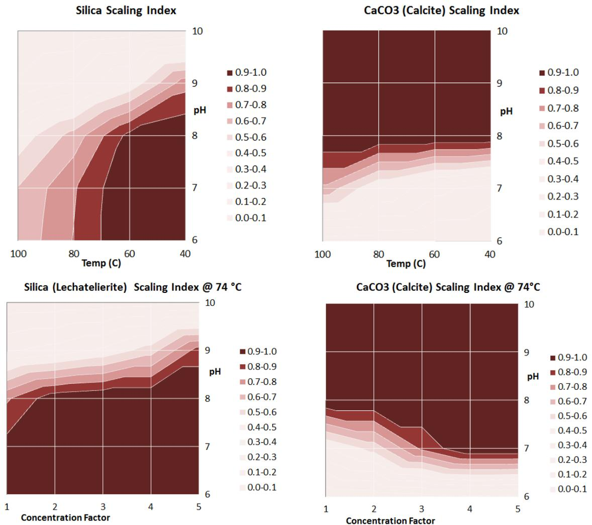
**Figure 1. Scaling tendency indices for silica (left column) and calcite (right column) for the injection brine at Tuscarora as a function of temperature (top row) or concentration factor (bottom row). Existing conditions:  $T = 74\text{ }^{\circ}\text{C}$ ,  $\text{pH} = 6.6$ , Conc. factor = 1. Scaling potential increases as the index approaches unity. (OLI Software)**
