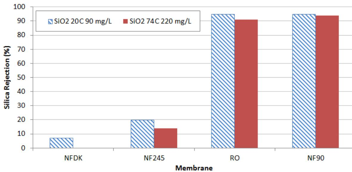
**Figure 4.** Silica rejection for simulated Tuscarora makeup water (blue stripes) and Tuscarora injection brine (red bars). Tests run at 150 psi to match the injection brine pressure. The NaCl pre-compaction test was operated at 300 psi. Cross flow was 1 LPM and membrane area 139 cm<sup>2</sup>.
