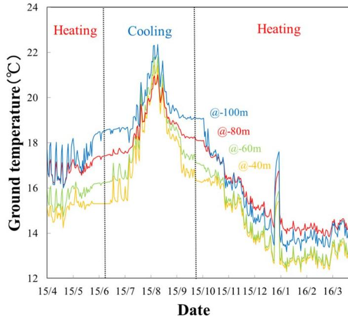
Figure 4. Change of ground temperature at -40 m, -60 m, -80 m, -100 m
