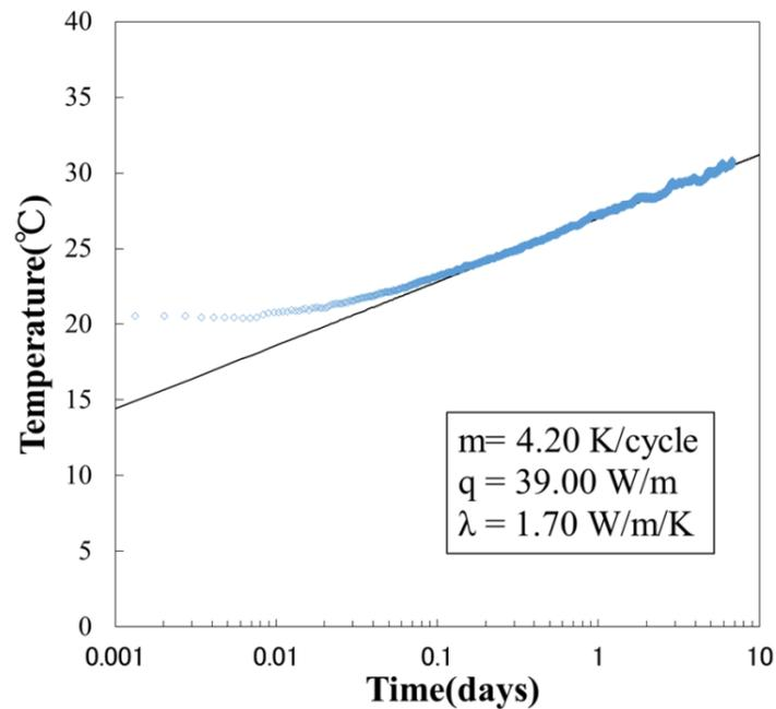
**Figure 6. Result of graphical method**
