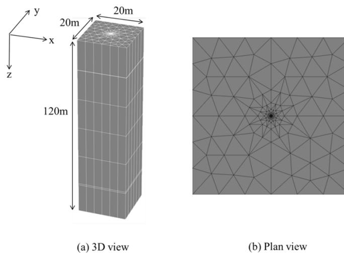
**Figure 7. Numerical model of single U-tube BHE**
