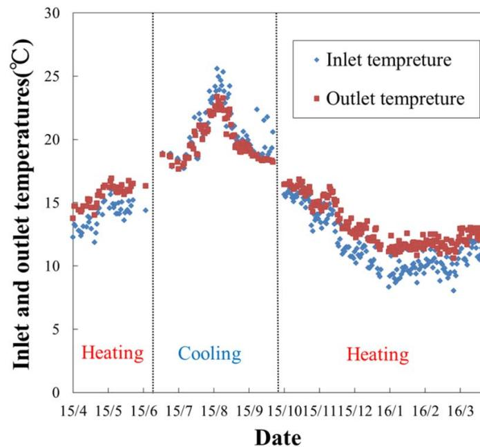
**Figure 3. Change of inlet temperature and outlet temperature during operation**
