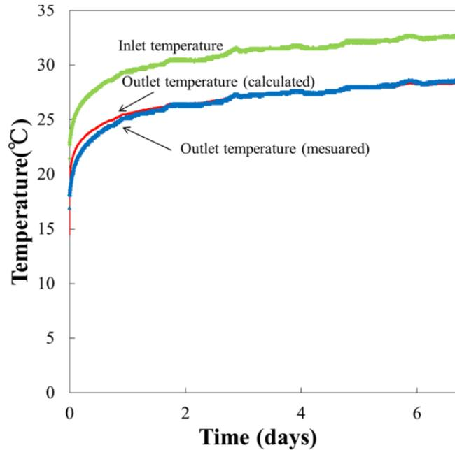
Figure 8. Result of history matching for single U-tube BHEs
