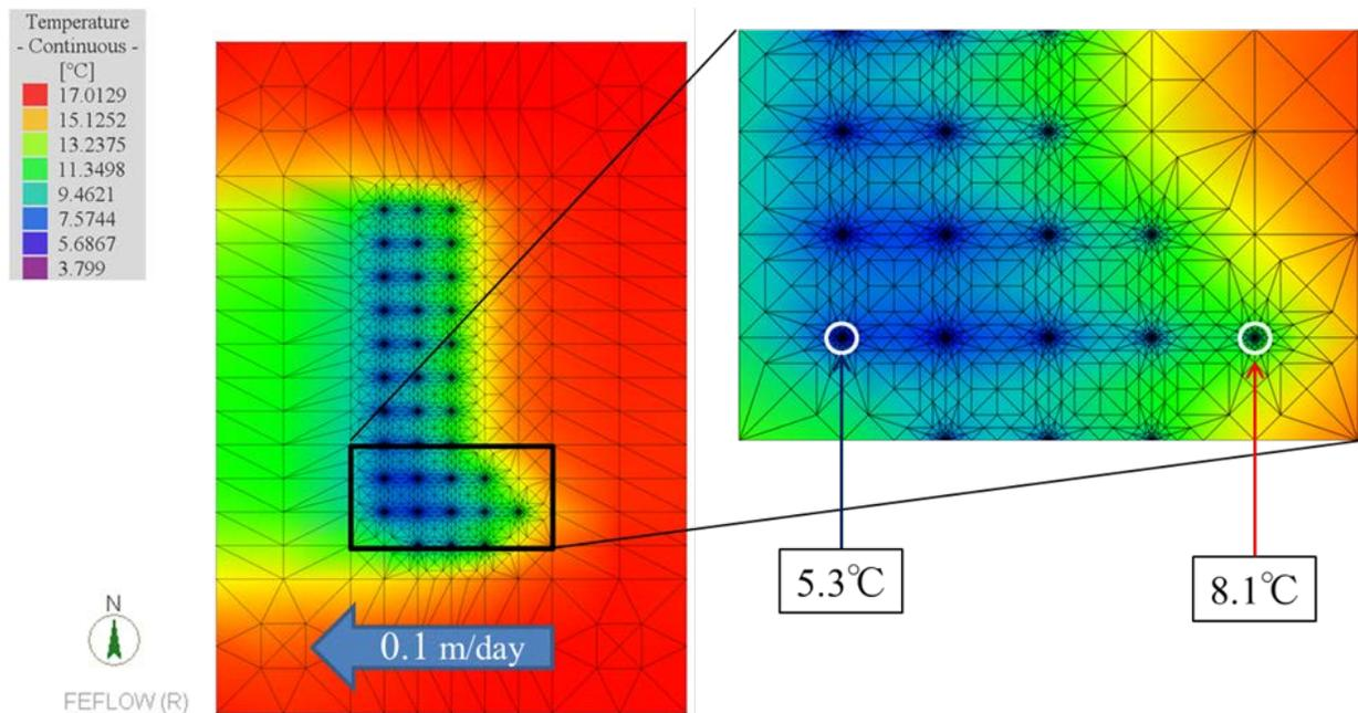
**Figure 13.** Distribution of ground temperature at -80 m at 10 years later
