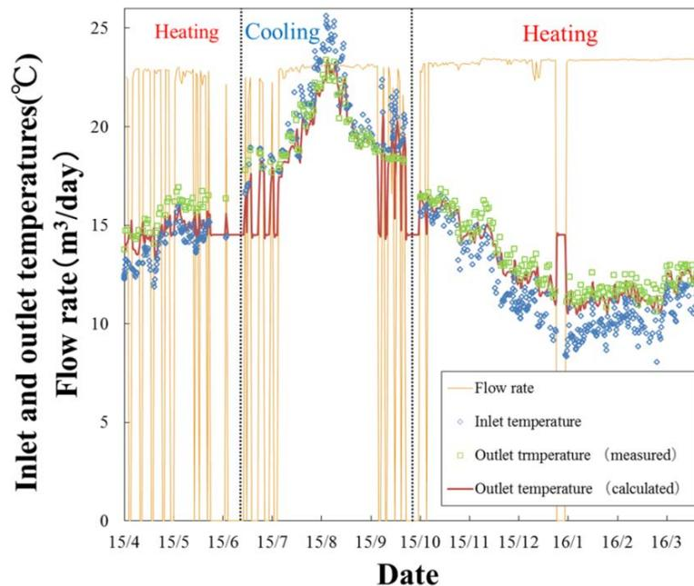
**Figure 10. Result of history matching of outlet temperatures for the borehole field**
