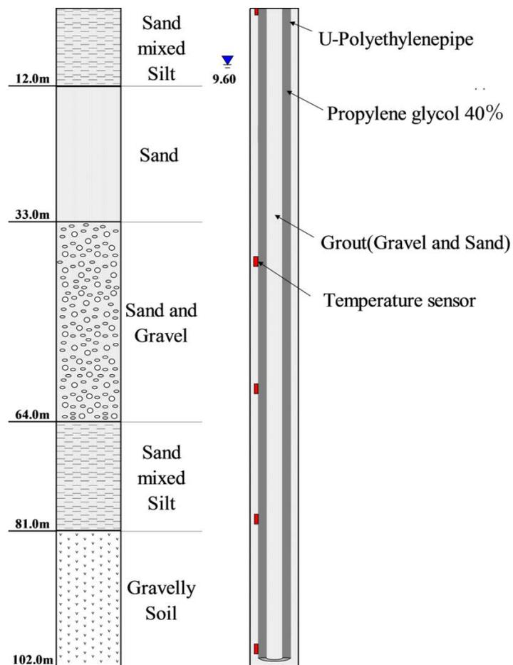
Figure 2. Geological column and well completion
