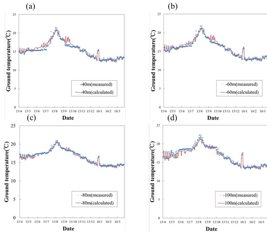
Figure 11. Result of history matching of ground temperatures, (a) -40 m, (b) -60 m, (c) -80 m, (d) -100 m
