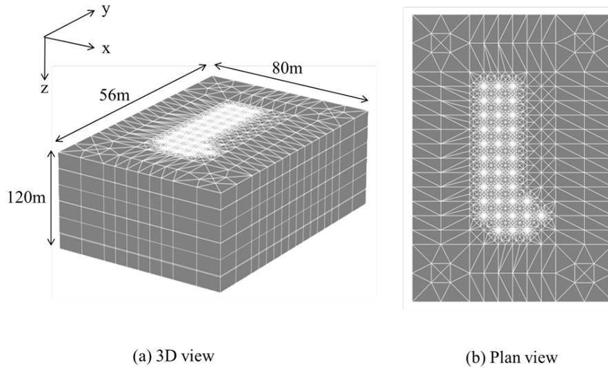
**Figure 9. Numerical model of the borehole field**
