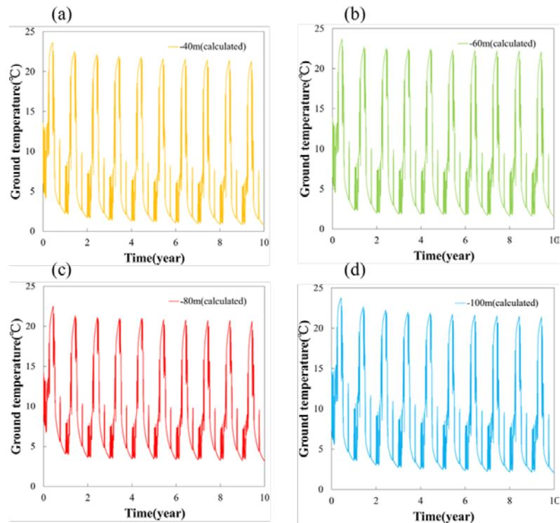
**Figure 12.** Result of future prediction of ground temperature (a) -40 m, (b) -60 m, (c) -80 m, (d) -100 m
