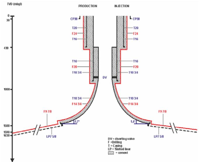
Figure 10. GDH doublet (sub) horizontal well profiles.
