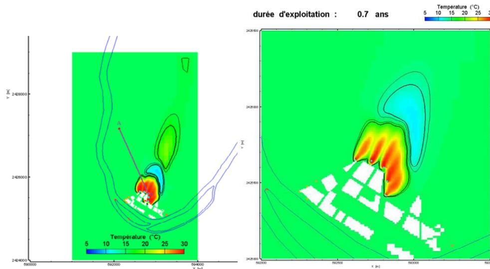
**Figure 18.** Shallow geothermal. Heat and Cold imbalance. Hot plume tracking.
