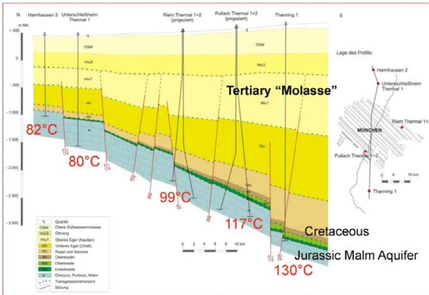
Figure 6. Geological cross section Munich Area N-S. (source: Erdwerk).
