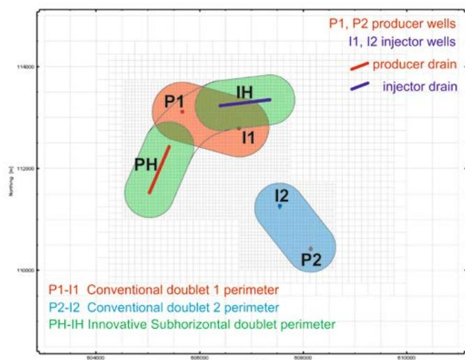
Figure 11. Conventional (deviated) vs innovative (subhorizontal drains) doublet well locations (reservoir impacts).
