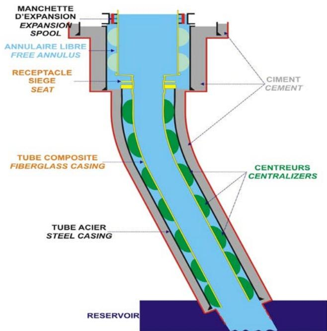
Figure 15. Anti-corrosion fiberglass lined well design.
