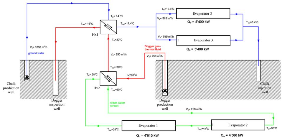
Figure 14. Preheating of shallow ground water (from 14 to 17.4°C) via direct heat exchange with deep geothermal water (Dogger reservoir) (Source: Friothersm, 2009).
