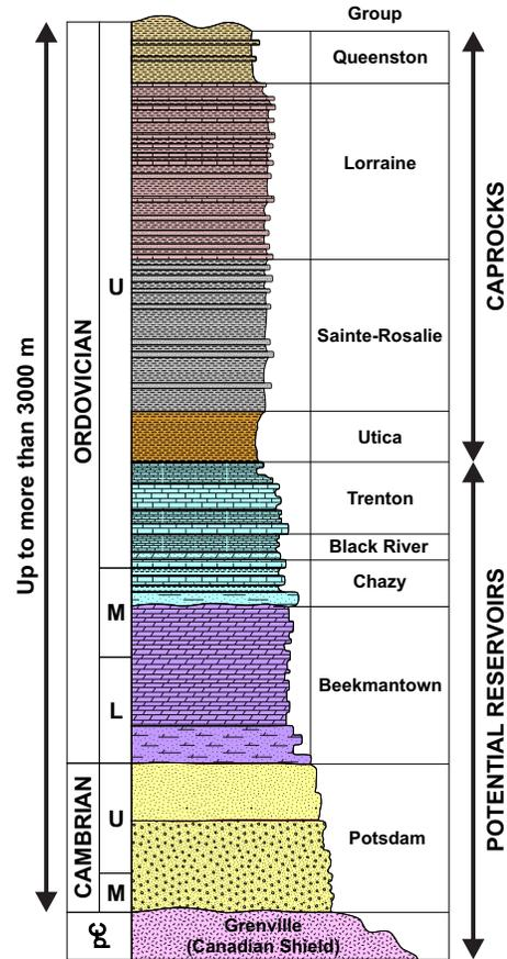
**Figure 3.** Simplified stratigraphic column of the SLL basin sedimentary sequence. Thickness of the sedimentary sequence is up to 3000 m in the deeper part of the basin. Modified from Comeau *et al.* (2013).
