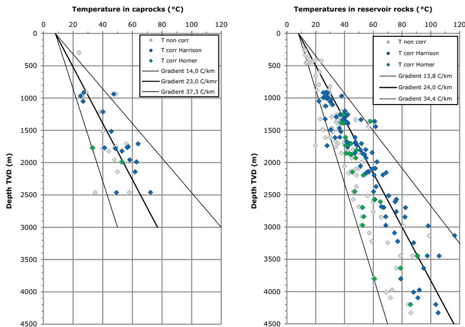
**Figure 4.** BHT data in caprocks (left) and in reservoir rocks (right) from oil and gas exploration wells in the SLL basin. The dashed lines represent the approximate minimum and maximum geothermal gradient of the corrected temperatures. The solid line shows the maximum gradient of the data corrected with Horner corrections.
