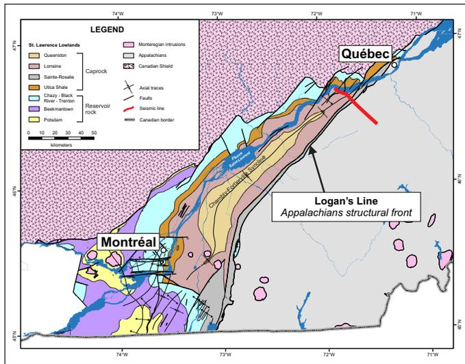
**Figure 1.** Geological map of the SLL basin (MRNF, 2008; Comeau *et al.*, 2013). The red line shows the location of seismic profile M-2001 (Figure 2). The yellow dots indicate the wells where heat flow measurements have been performed (Misener *et al.*, 1951; Saull *et al.*, 1962; Fou, 1969).
