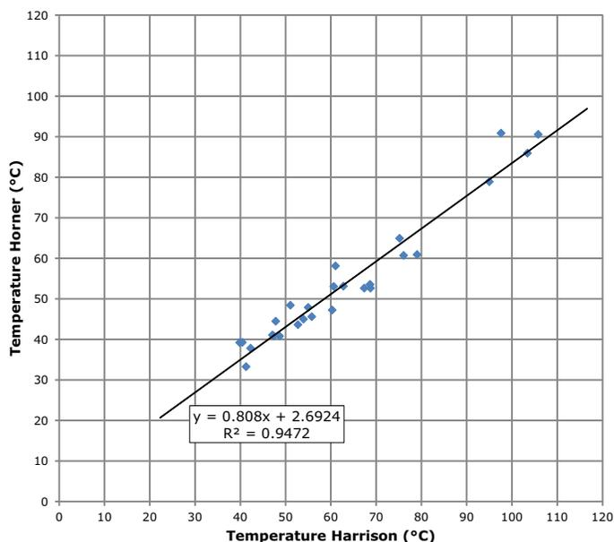
**Figure 5.** Difference between temperatures corrected with Harrison and Horner corrections.
