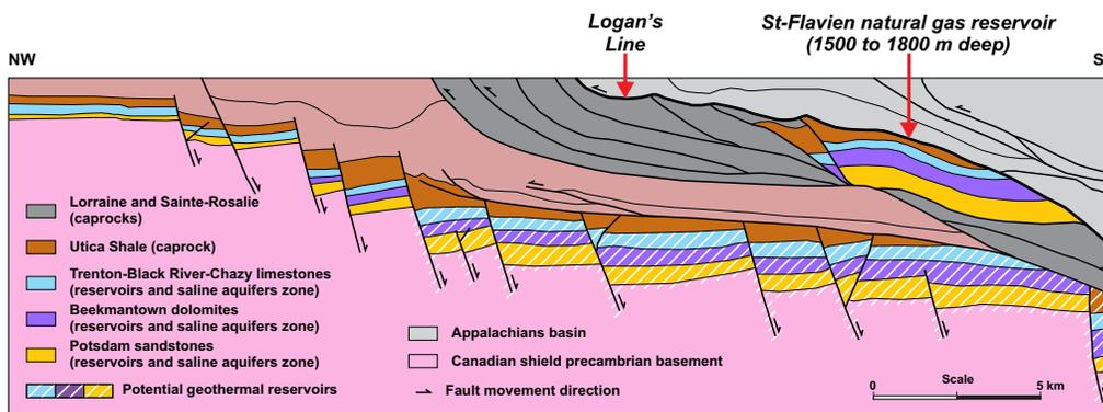
**Figure 2.** Interpreted cross-section based on M-2001 seismic profile (Castonguay *et al.*, 2010) showing the potential geothermal reservoirs. Location of the seismic line is given in Figure 1.
