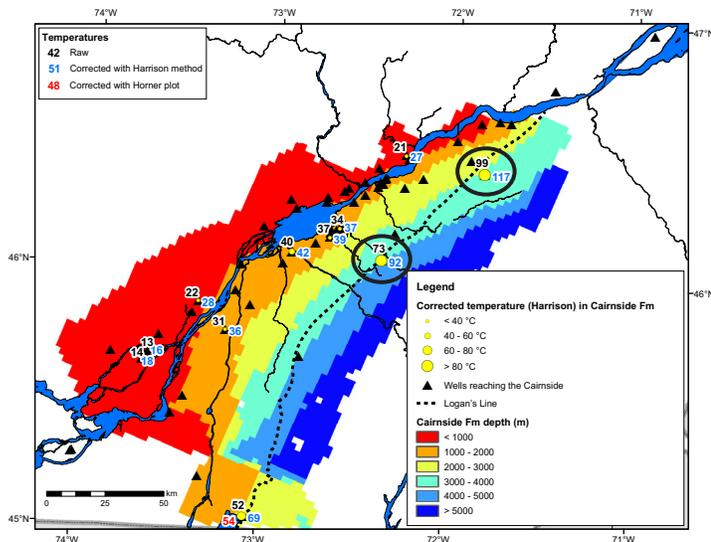
**Figure 6.** Depth of the top of the Cairnside Formation and temperature data that intersected this unit. Black circles indicate the wells in which temperature is the higher.
