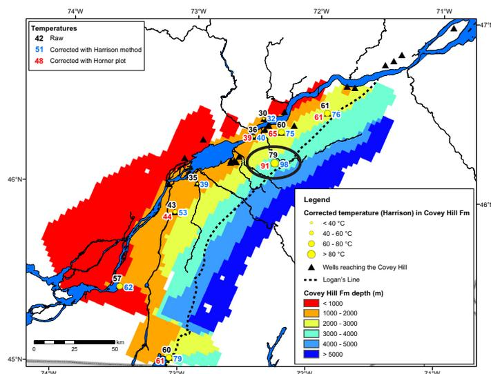
**Figure 7.** Depth of the top of the Covey Hill Formation and temperature data that intersected this unit. The black circle indicates the well in which temperature is the higher.
