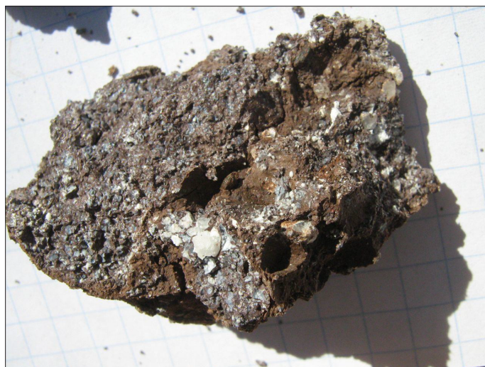
Figure 5B. Photograph of rock sample from Paisley production well SVE-1 at a depth of approximately 1100 feet. (Blue squares are 1/4 inch.)
