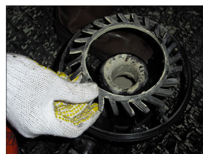
Figure 10. Water Distribution Spray Nozzle Post Injections 2013.
