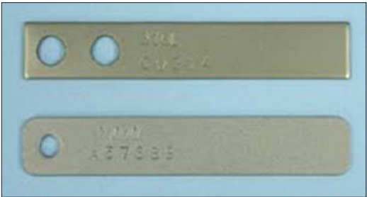
Figure 2. Strip Corrosion Coupons.
