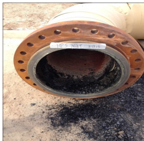
Figure 7. High Pressure steam pipe 2015 after the Scale inhibitor treatment.
