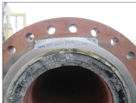
Figure 6. High Pressure steam pipe 2013 Prior to the Scale inhibitor treatment.
