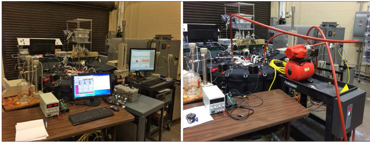
Figure 1. Fully assembled test systems (left) and heating by circulating hot water (right).
