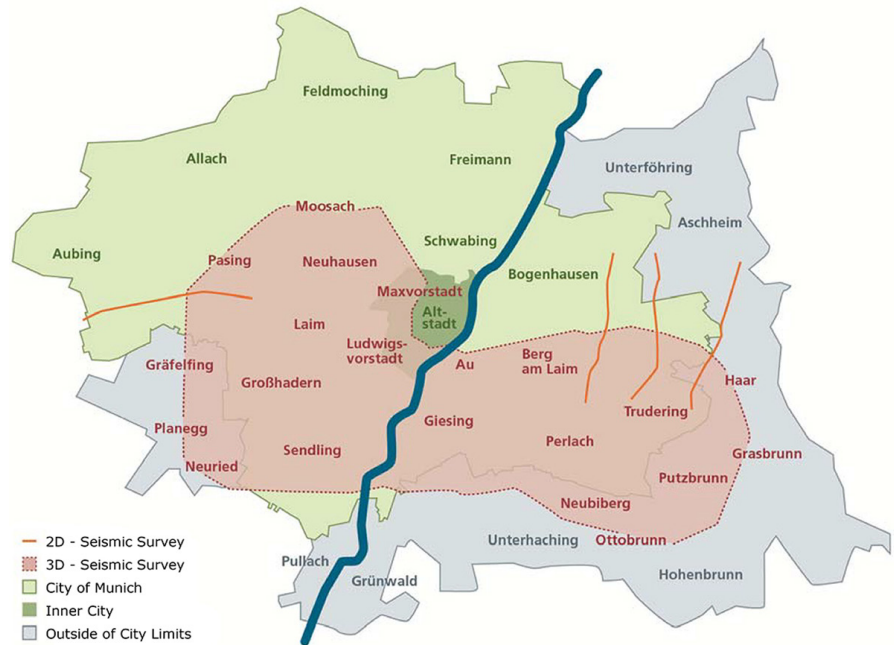
Figure 8. Overview of 3D Seismic survey area and existing 2D Seismic lines in relation to Munich city districts. Adapted from SWM original in German. Copyright SWM GmbH.
