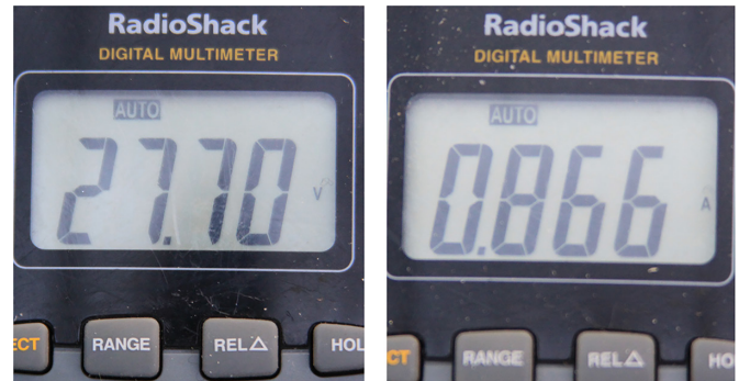
Figure 6. Hveragerdi outdoor thermoelectric generator short circuit voltage (left) and open circuit current (right).
