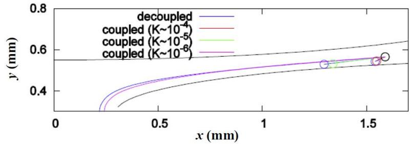
Figure 4. Particle trajectories in the single particle deposition problem using the initial particle position (X,Y)=(1.59, 0.565) for three permeability values (1.1718×10<sup>-4</sup> mm<sup>2</sup>, 1.1718×10<sup>-5</sup> mm<sup>2</sup>, 1.1718×10<sup>-6</sup> mm<sup>2</sup>). The initial particle position is denoted by a black circle, and the upper and lower curves around the channel represent the porous boundary.
