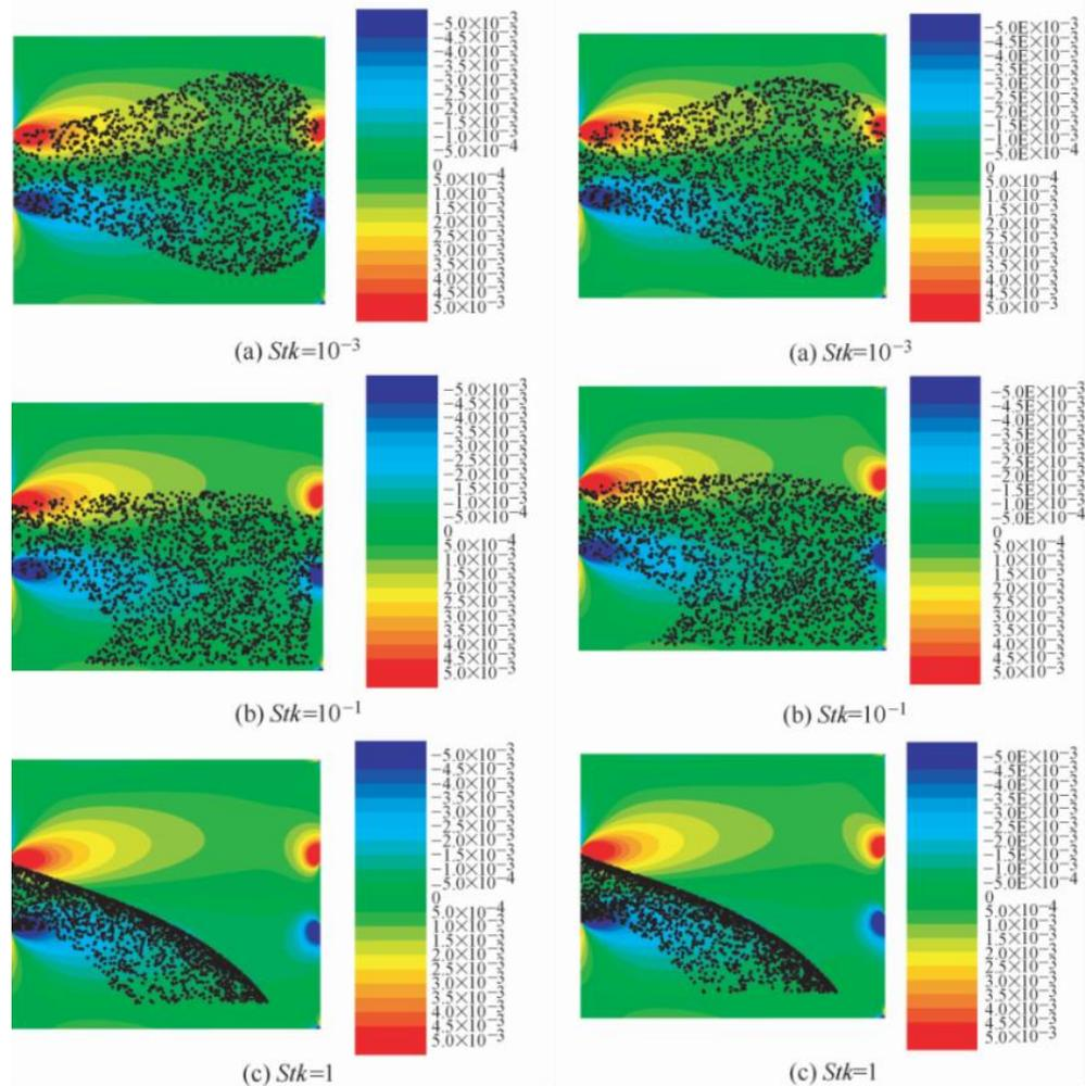
**Figure 8.** Particles distribution assuming different Stokes numbers (a) Without natural convection; (b) With natural convection ( $Ra=10^4$ ).
