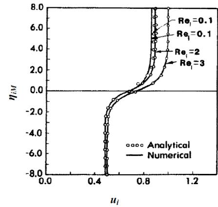
**Figure 7.** Velocity distributions at the interface region between two different porous media ( $u_i$ , convection velocity, m/s;  $\eta_{in}$ , non-dimensional coordinate for the upper porous media).
