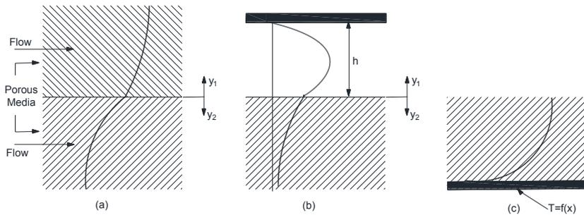
**Figure 6.** The interface region (a) between two different porous media (b) between a porous and a fluid region (c) between an impermeable media and a porous media.
