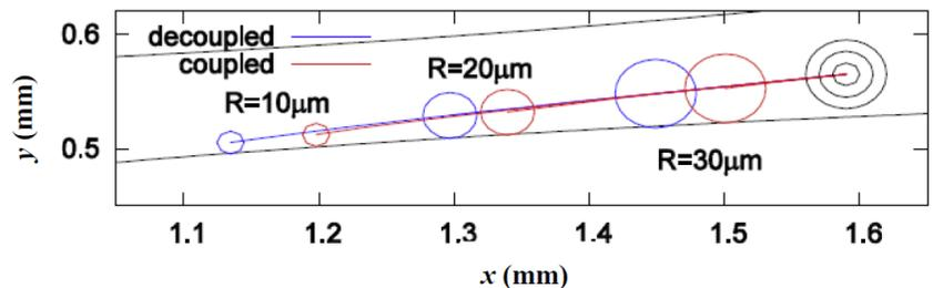
Figure 5. Effects of particle size on particle deposition. Three particles of different radius (10, 20 and 30µm) are initially located at the same position, denoted by black circles. In the case, the permeability of the porous media is  $K_p=1.1718 \times 10^{-5}$  mm<sup>2</sup>.
