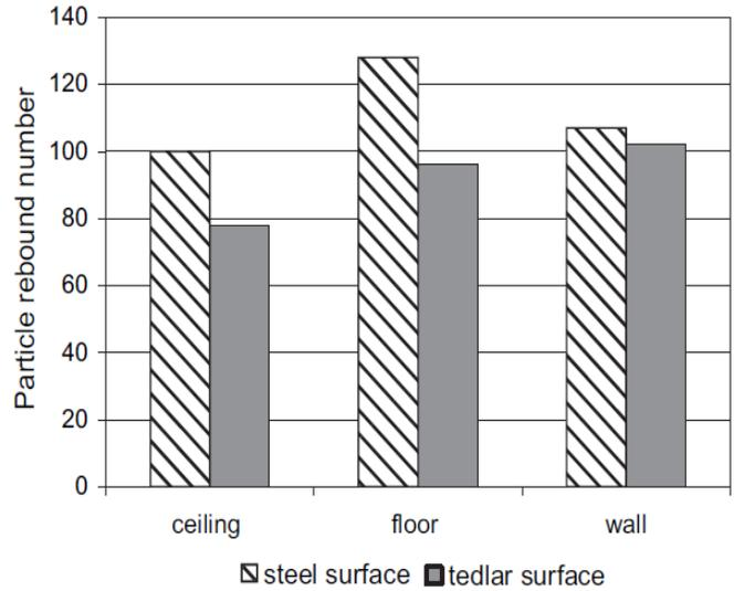
Figure 3. Particle rebound number (Jiang et al., 2010).
