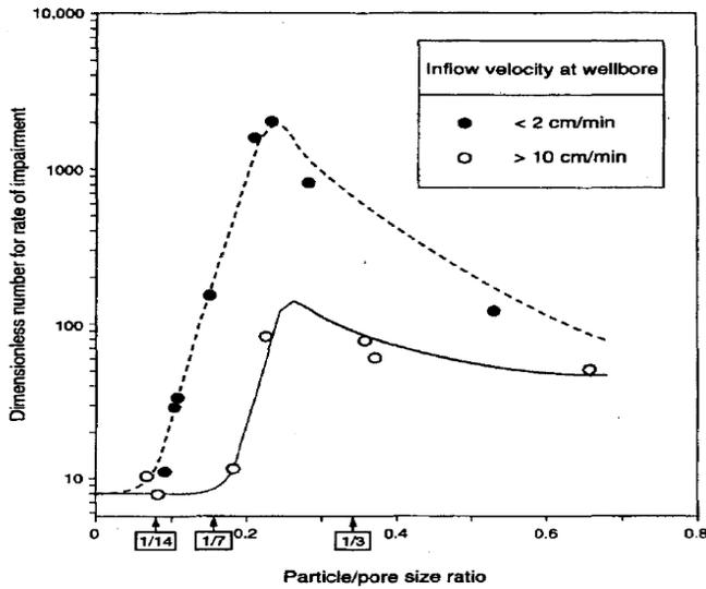
Figure 2. Impairment rate as a function of particle/pore size ratio (Oort et al., 1993).
