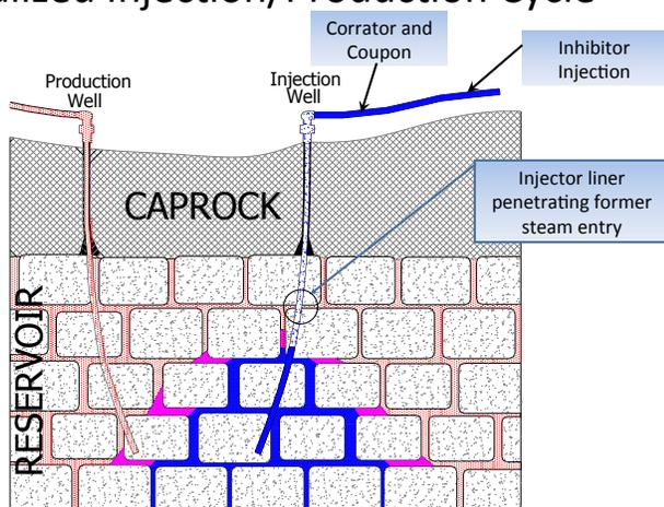
Figure 1. Idealized injection/production cycle.
