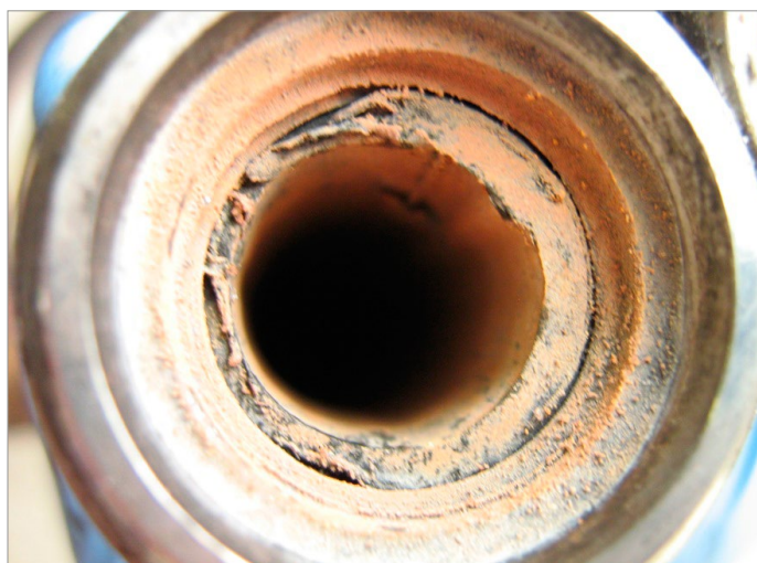
Figure 3. End coupling of the heat exchanger with the treatment.
