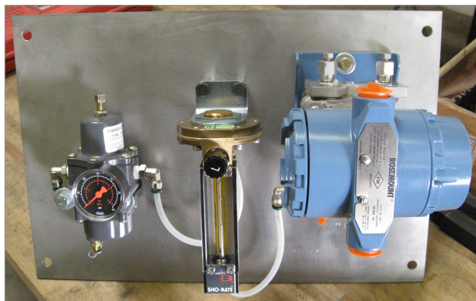
Figure 2. Example of bubbler panel.
